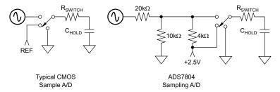
Figure 10. Comparison of Input Structures
