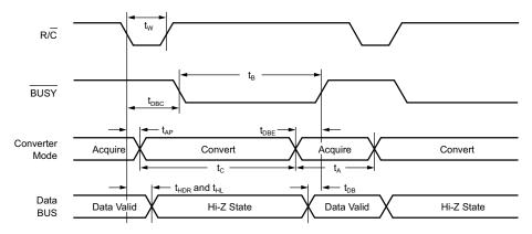
Figure 13. Convert Mode: R/C Pulse LOW — Outputs Enabled After Conversion
