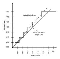
Figure 3. Positive Gain Error
