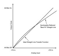
Figure 6. Integral Nonlinearity Referred to Best-Fit Straight Line
