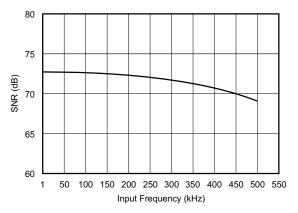
Figure 8. SNR vs Input Frequency for ADS602
