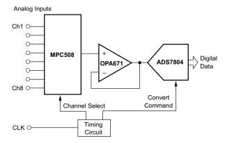
Figure 9. Traditional Analog Multiplexing System
