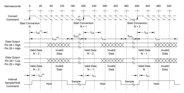
Figure 14. Basic Conversion Timing
