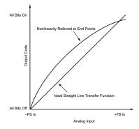
Figure 5. Integral Nonlinearity Referred to Inputs
