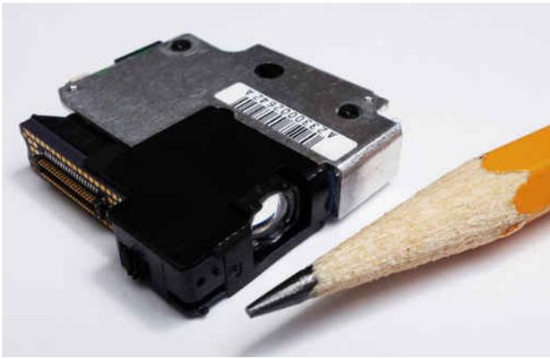
**Figure 6.** An ultra-compact DLP2010 (0.2-inch 854 x 480 resolution) optical module with approximate dimensions of 30 mm by 30 mm by 6 mm.
