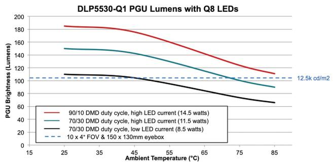
**Figure 11.** PGU brightness as a function of temperature, DMD duty cycle and LED current
