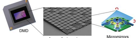
Figure 1. Digital Micromirror Device (DMD).
