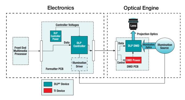
Figure 6. Typical DLP display system block diagram.
