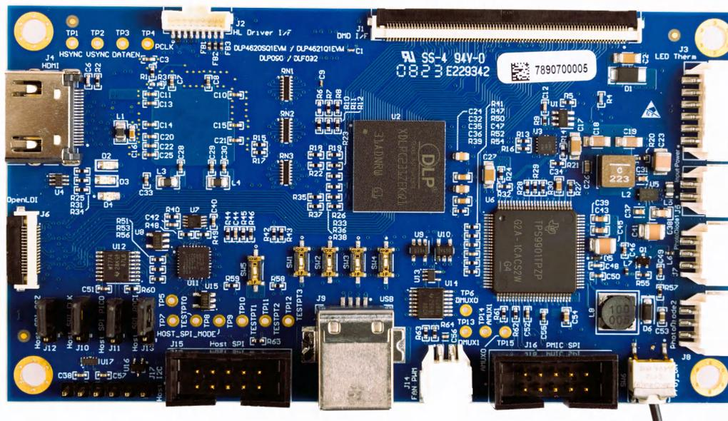
**Figure 2-3. DLPC231SQ1EVM Controller PCB**
