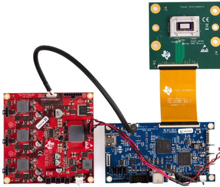
**Figure 3-2. DLP4621Q1EVM EVM Cable Connections**
