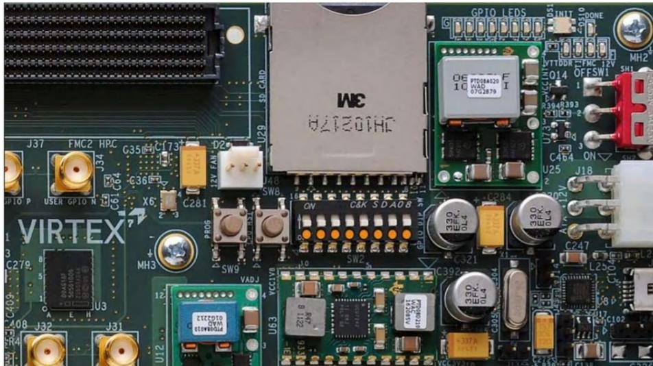
**Figure 4-10. GPIO Dip Switches (VC707)**
