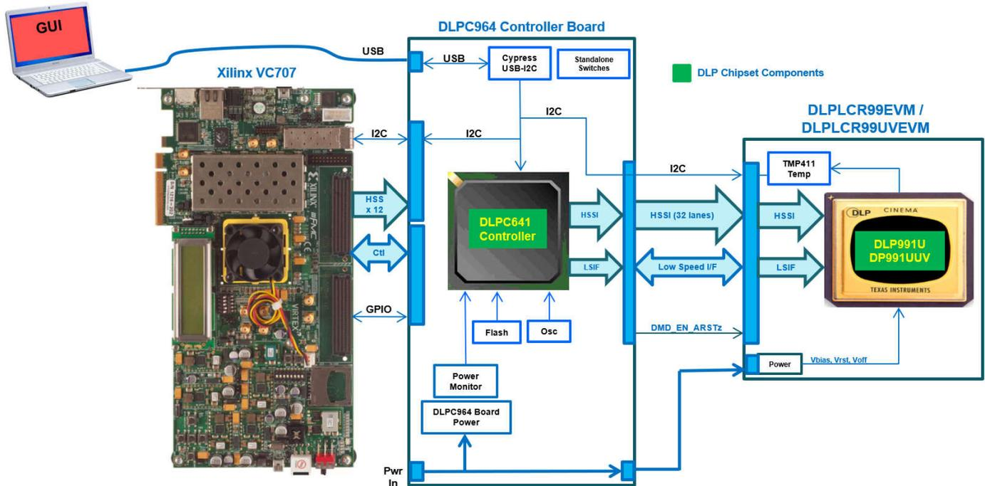
Figure 1-2. DLPLCR964EVM Hardware Components
