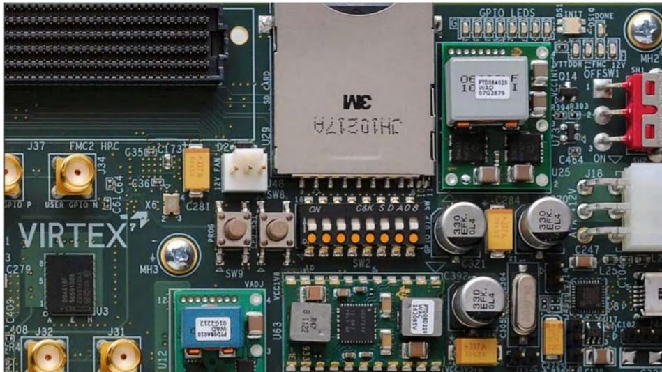
**Figure 3-20. GPIO Dip Switches (VC707)**
