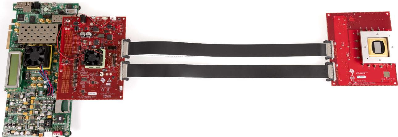
Figure 2-6. Fully Assembled DLPLCRC964EVM with AMD EVM
