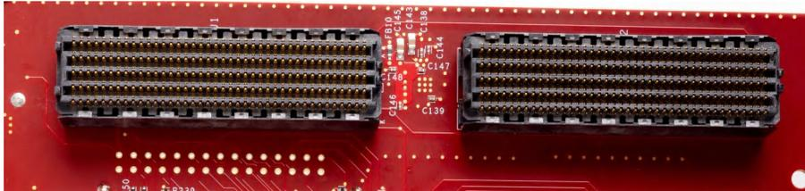
Figure 2-4. DLPLCRC964EVM Female HPC FMC Connector
