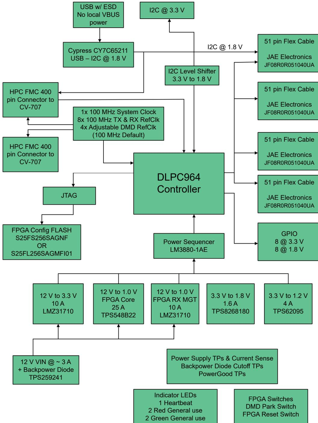
Figure 1-1. DLP LightCrafter DLPC964 EVM Block Diagram
