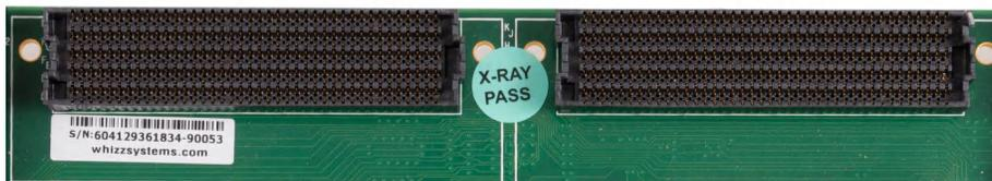
Figure 2-5. AMD EVM Female HPC FMC Connector
