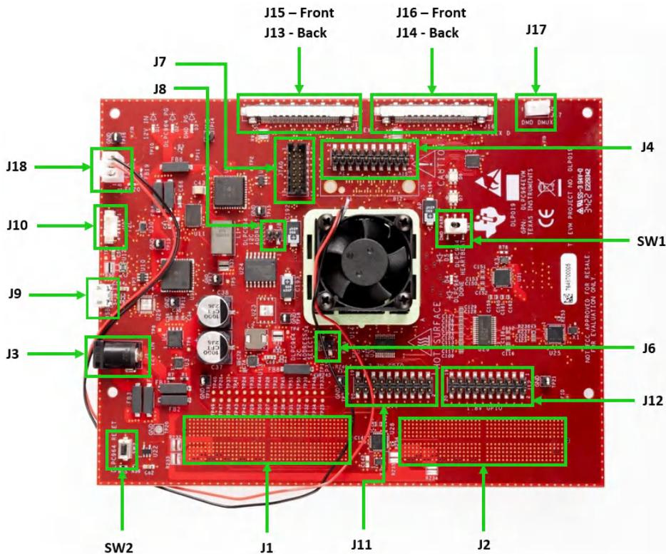
Figure 2-1. DLPLCRC964EVM Connectors (Top View)
