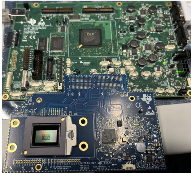
Figure 2-1. EVMs Connected
