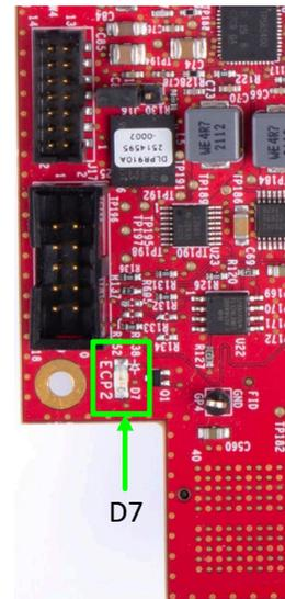
**Figure 3-5. DLP LightCrafter DLPC910 EVM LEDs (Top View - Lower Left)**
