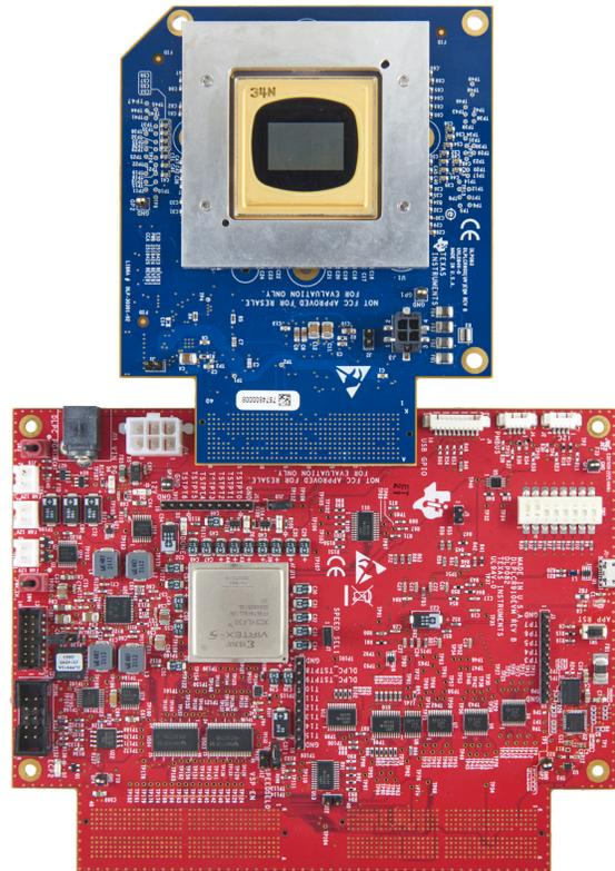
Figure 3-14. Assembled DLPLCRC910EVM with DLPLCR90XEVM or DLPLCR90XUVEVM (without cable)
