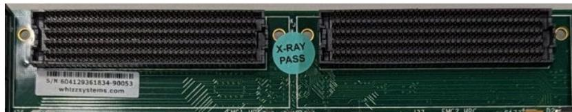
**Figure 3-19. AMD Xilinx VC-707 Female HPC FMC Cable Connectors**
