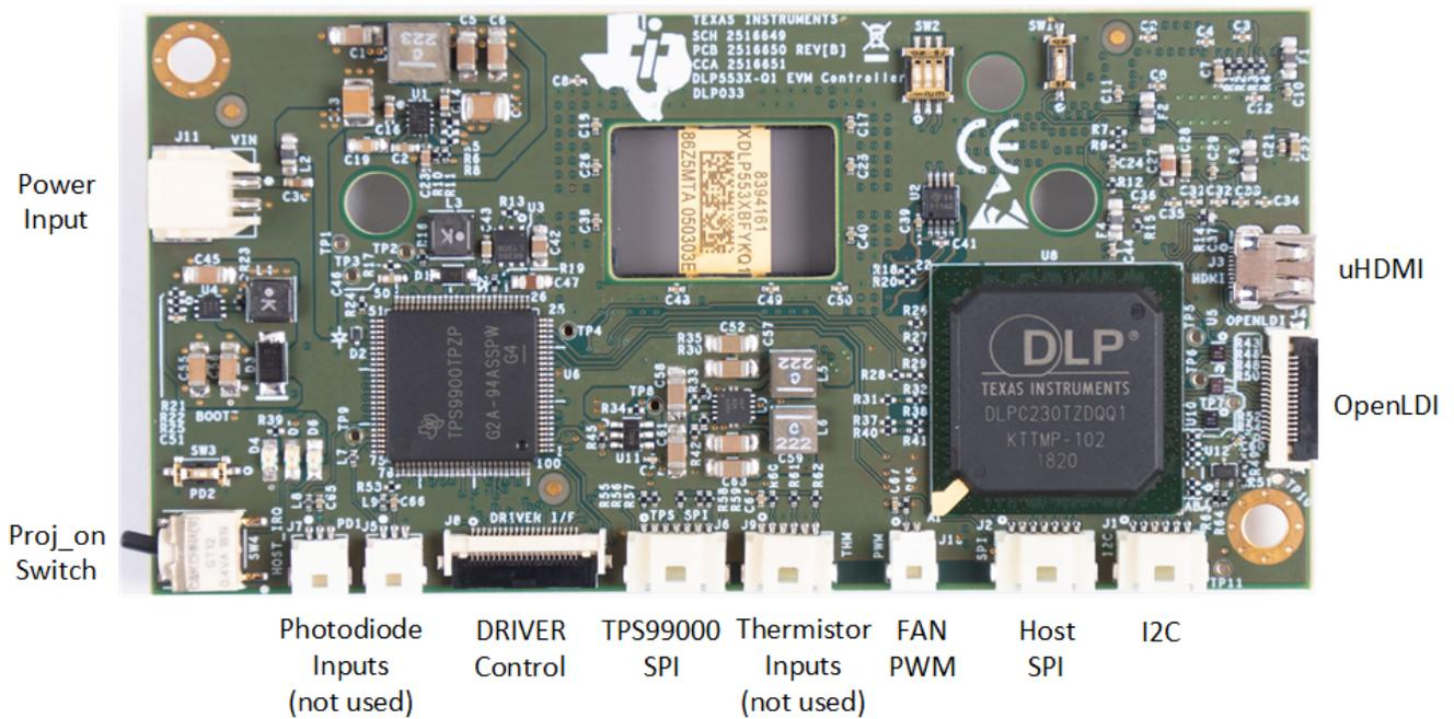
Figure 2. EVM Controller PCB
