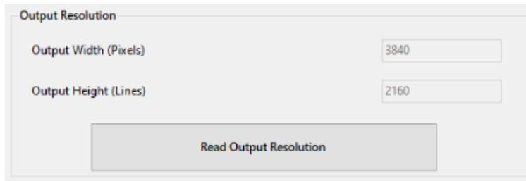
When the output resolution information has been read from the projector system, all other GUI elements that are relevant for the next step of action are enabled.
