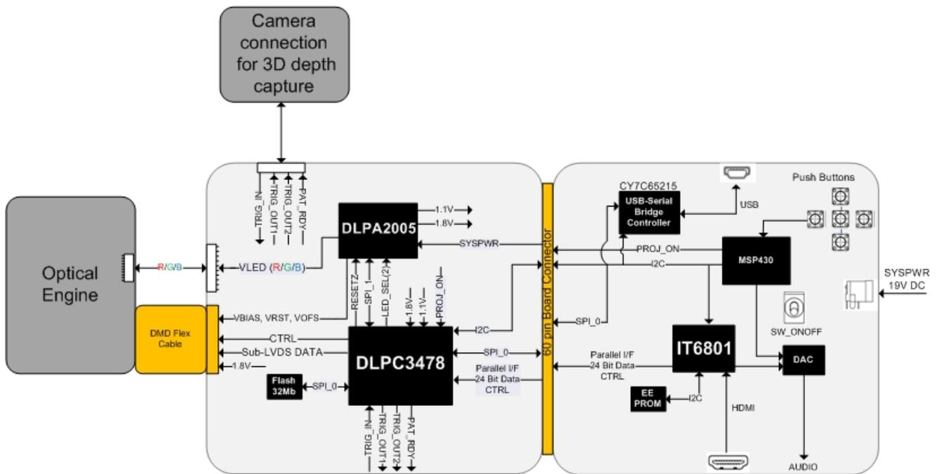
Figure 2. DLP3010 Light Control EVM Block Diagram
