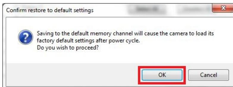
**Figure 4-6. Confirm Factory Camera Settings in FlyCap2 Software**
