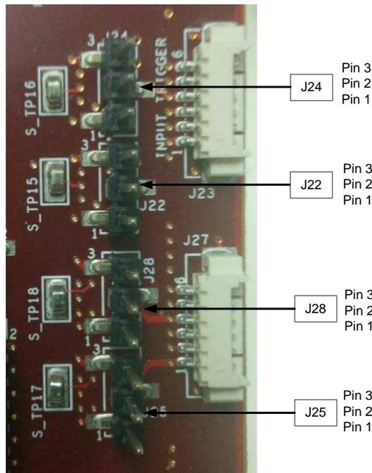
**Figure 1-10. DLP LightCrafter 9000 Trigger Voltage Level Selectors**
