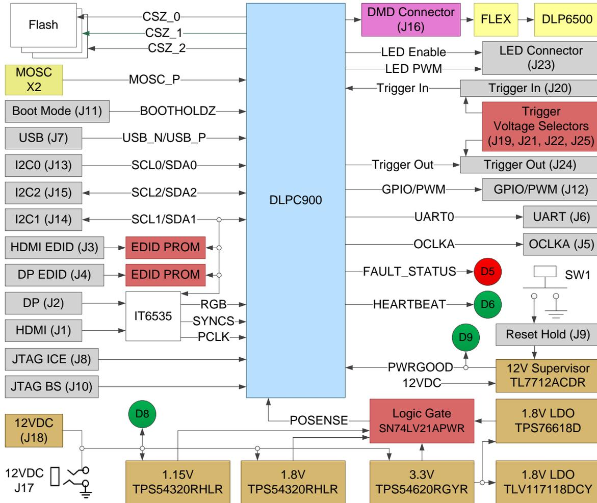
Figure 1-3. DLP LightCrafter 6500 EVM Block Diagram
