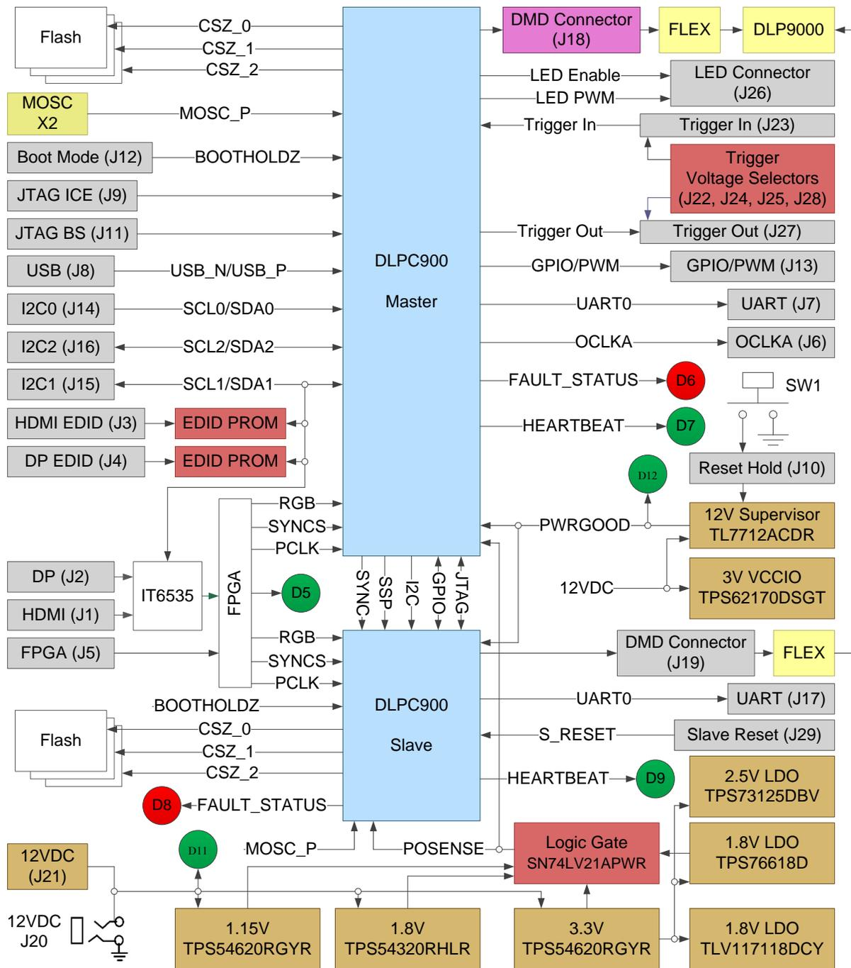
Figure 1-4. DLP LightCrafter 9000 EVM Block Diagram
