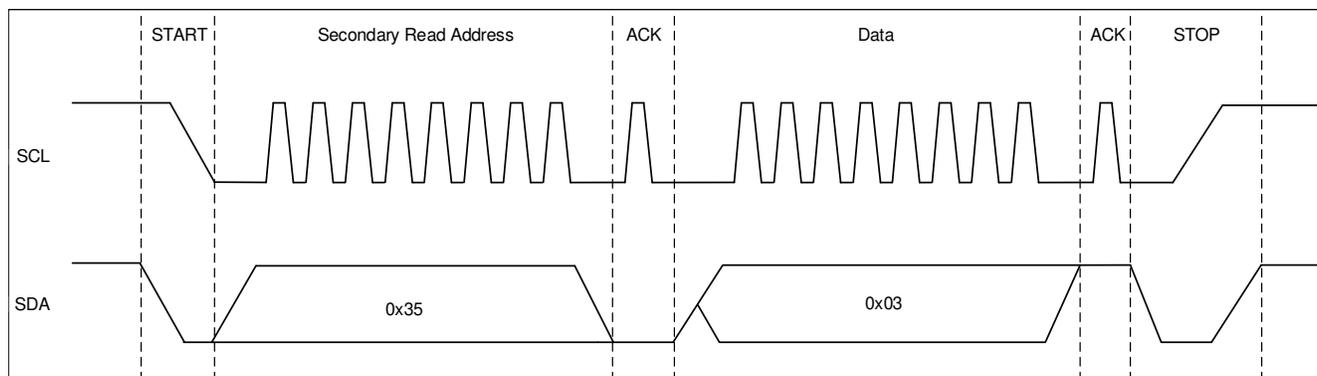
**Figure 1-2. I<sup>2</sup>C Read Data Waveform Diagram**
