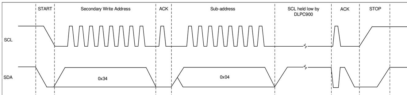
**Figure 1-1. I<sup>2</sup>C Read Command Waveform Diagram**
