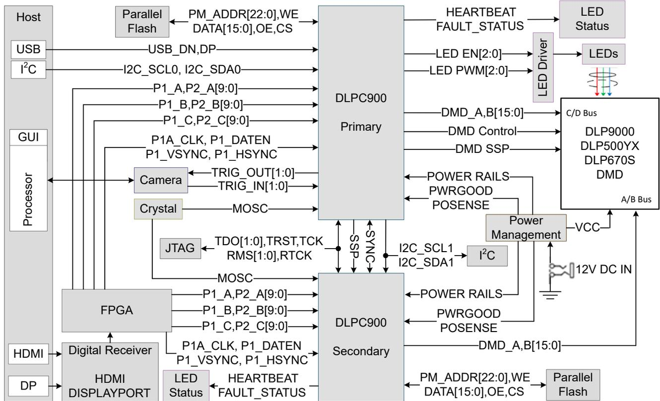
Figure 2-5. DLPC900 Dual Controller System Block Diagram
