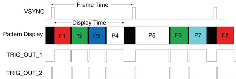
**Figure 2-8. Video Pattern Mode Timing Diagram Example**
