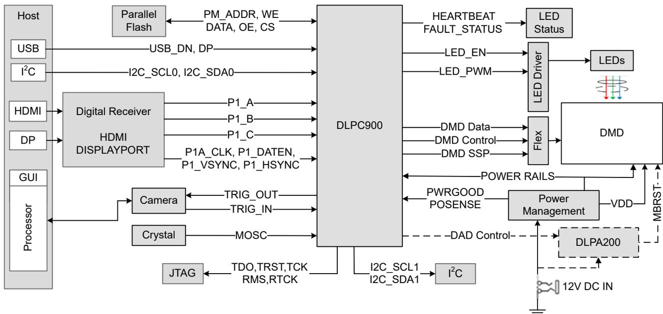
**Figure 2-4. DLPC900 Single Controller System Block Diagram**
