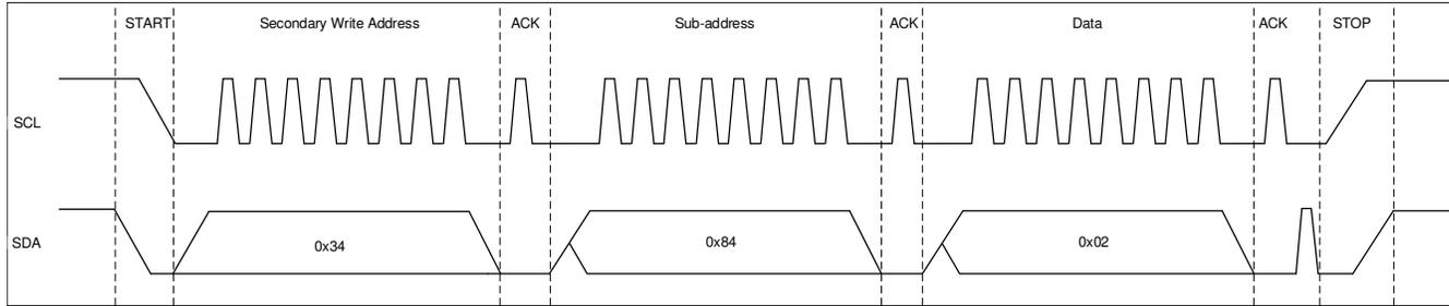
Figure 1-3. I<sup>2</sup>C Write Command Waveform Diagram
