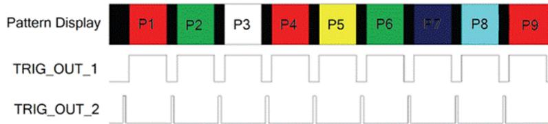
**Figure 2-9. Pre-Stored Pattern Mode Timing Diagram Example**
