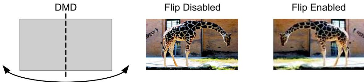
**Figure 2-1. Image Long-Axis Flip Example**
