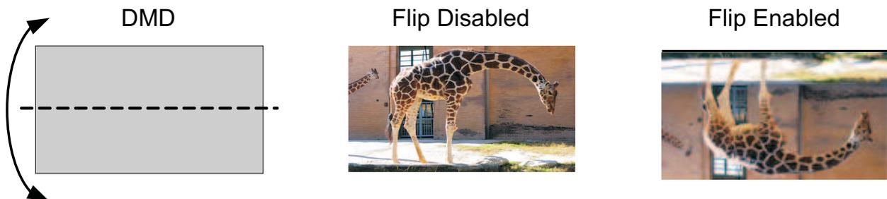
**Figure 2-2. Image Short-Axis Flip Example**
