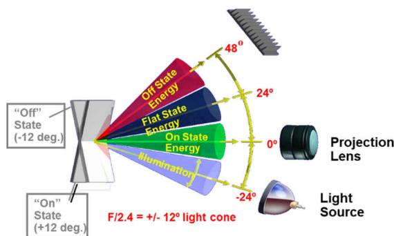
**Figure 3-1. Illumination Diagram of Standard DLP Projector**
