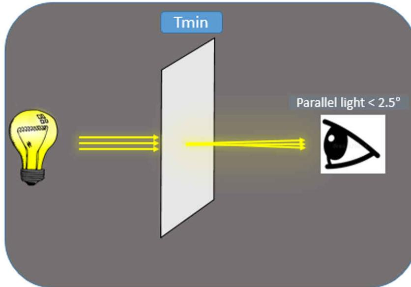
**Figure 2-4. T-min is the Amount of Specular Transmission of Incident Light When in the Translucent State**
