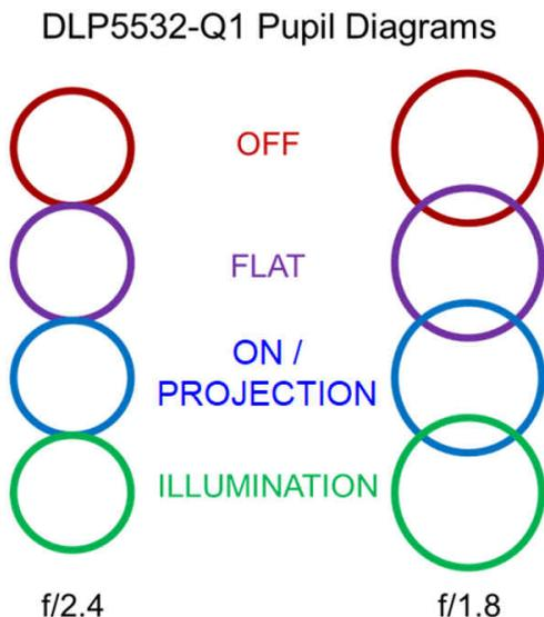
**Figure 3-2. Pupil Diagram of DLP5532-Q1 Projector at f/2.4 and f/1.8 Aperture Sizes**
