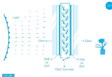
**Figure 2-1. PDLC Film in the Off State (no applied voltage)**
