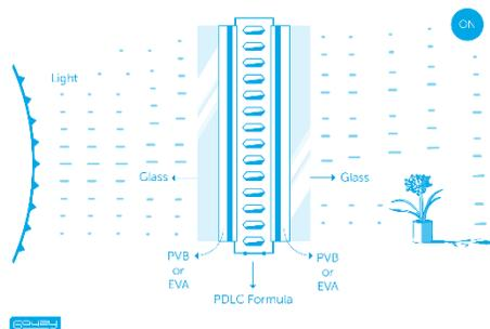
**Figure 2-2. PDLC Film in the On State (+48V applied)**
