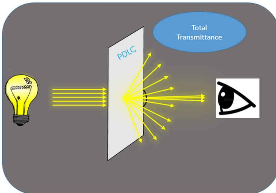
**Figure 2-5. T-total is Total Amount of Light (specular, diffused, and scattered) Transmitted When in the Translucent State**
