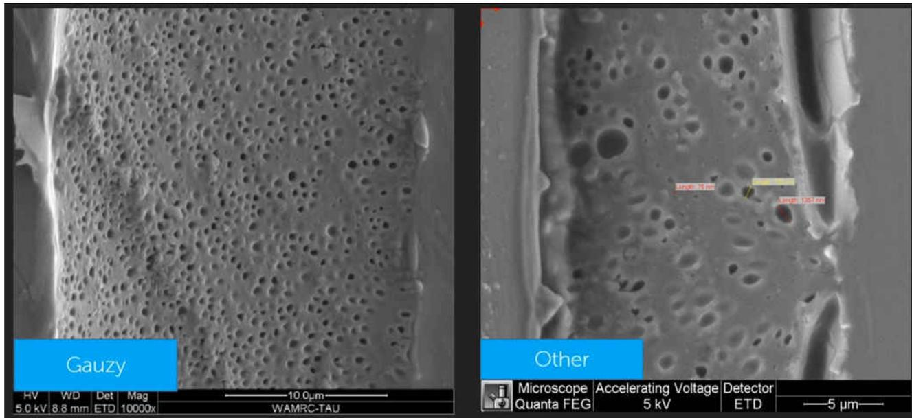
**Figure 2-3. Two Different PDLC Morphologies. The More Consistent the Size and Distribution of the Liquid Crystal Droplets, the Better the Optical Performance.**
