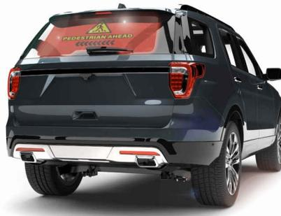
**Figure 1-1. V2V Communication Back Window Display**
