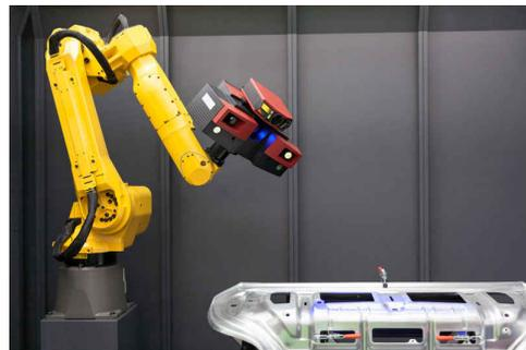
Figure 1. 3D Scanner Mounted on Robotic Arm
