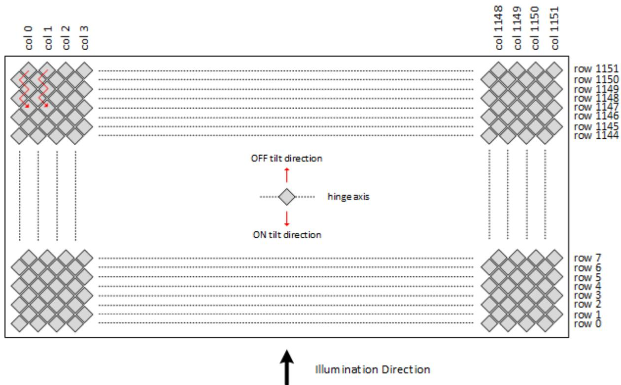
**Figure 1. 1.3 million micromirrors in a diamond pixel format**
