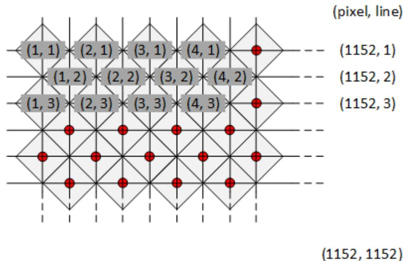
**Figure 7. 1152 x 1152 operating mode input to output mapping**
