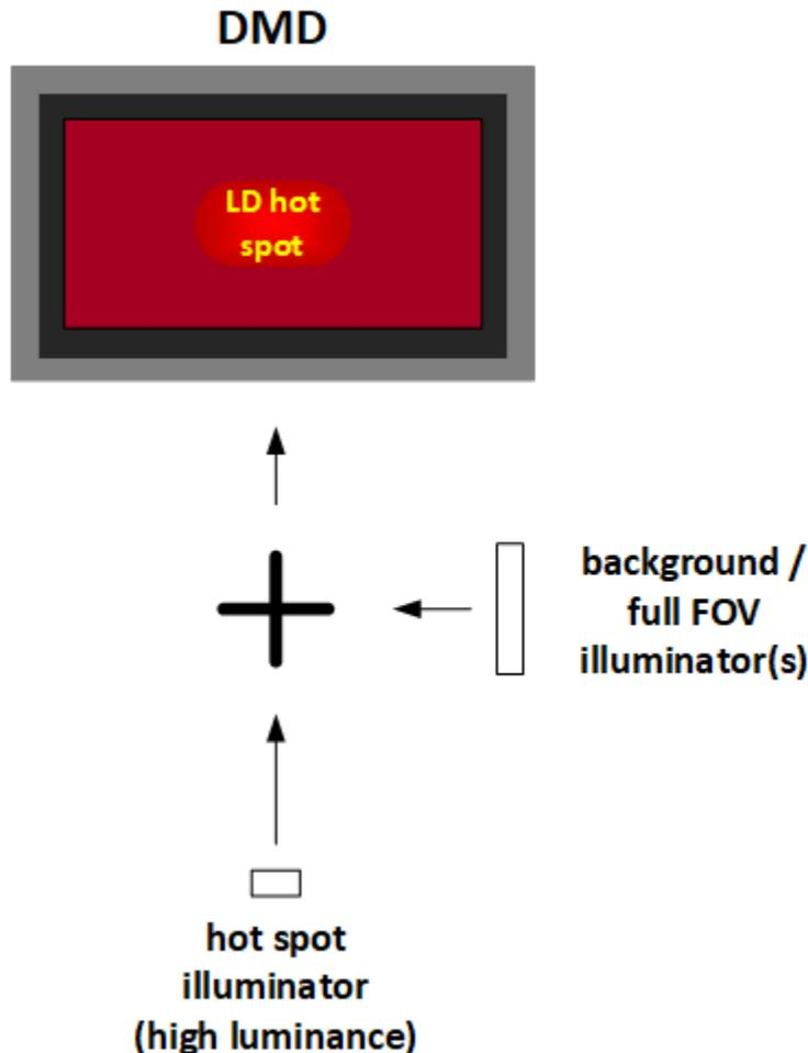
**Figure 20. High-luminance hotspot plus background illumination concept schematic**
