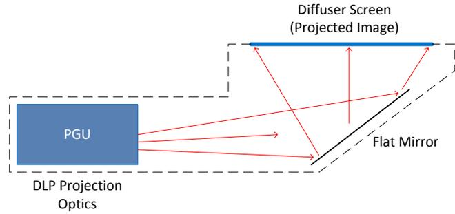
**Figure 11. Example PGU layout volume measurements**
