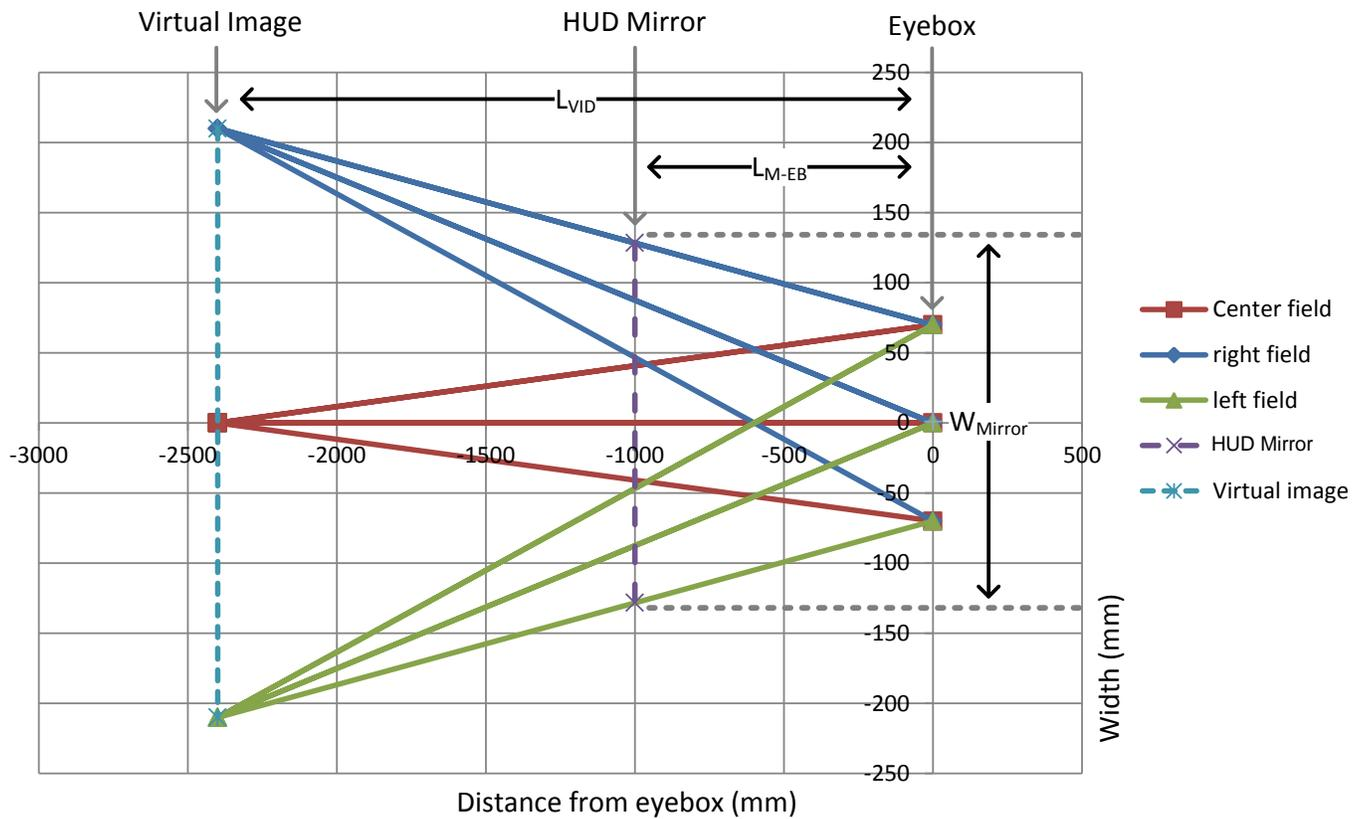
Figure 3. Width calculation of the primary mirror
