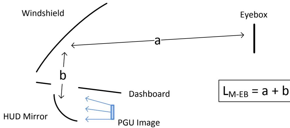
Figure 4. Distance from the eyebox to the primary mirror
