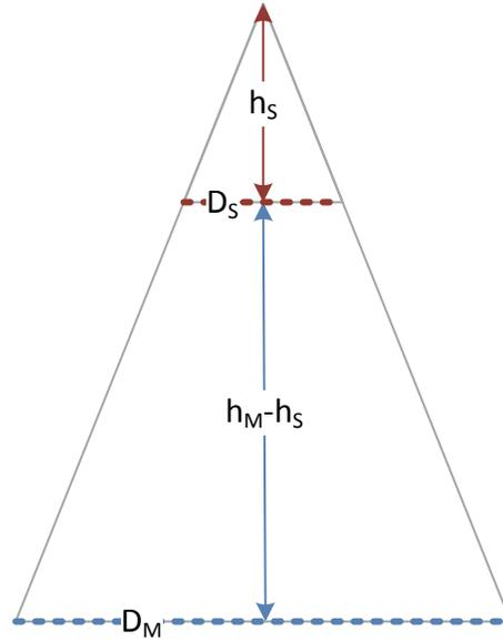
Figure 9. 2D representation of HUD volume pyramid diagonal
