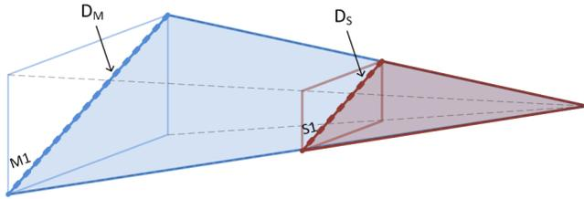
Figure 8. Diagonal area of the HUD volume pyramid
