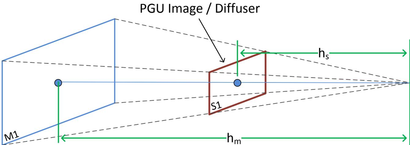
**Figure 7. Geometry of the primary mirror and diffuser screen**
