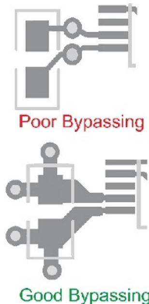
**Figure 3. Decoupling Capacitor Example**
