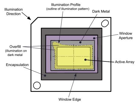
Figure 5. Optical Illumination Overfill
