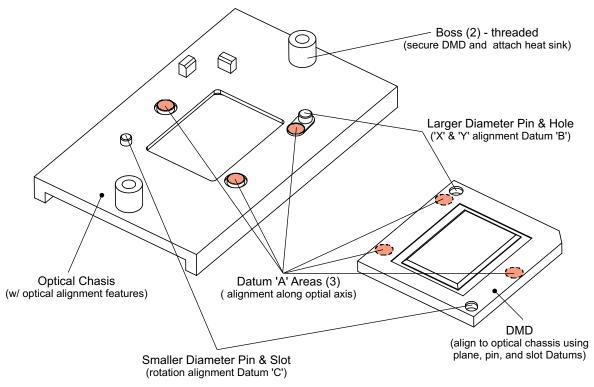
Figure 12. Optical Interface (Alignment) Features
