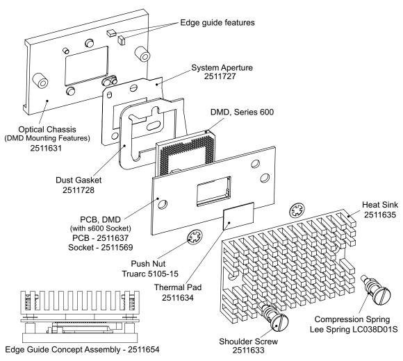
Figure 17. DMD Mounting Concept – Edge Guide
