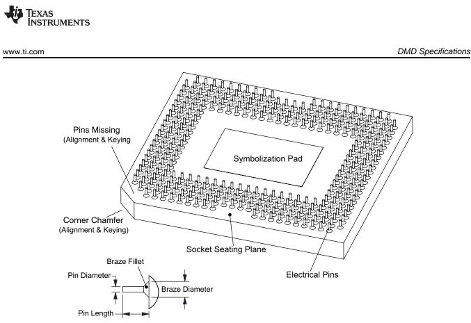
Figure 8. Electrical and Thermal Interface
