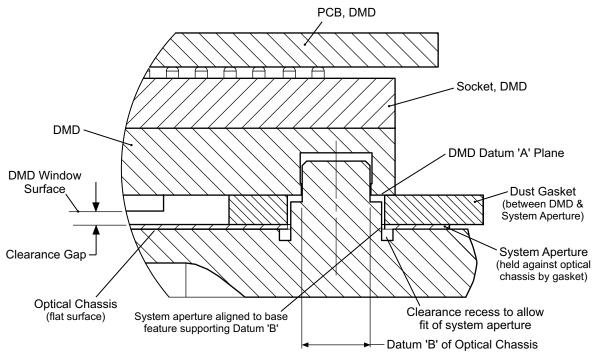
Figure 16. System Aperture and Dust Gasket
