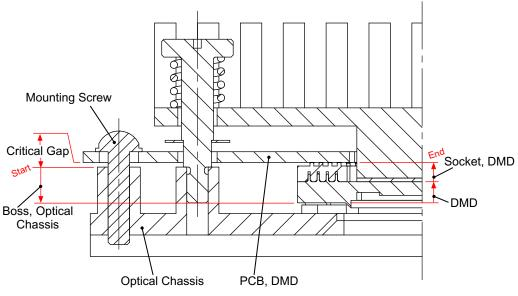
Figure 19. DMD-PCB Gap Analysis Schematic Diagram
