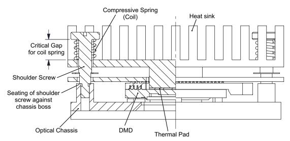
Figure 13. Heat Sink Mounting – Load Control by Design
