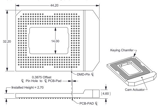
Note: DMD-Pin is not concentric with PCB-Pad
