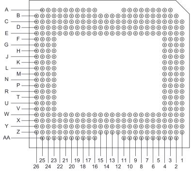
Figure 7. Pin Numbering Scheme
