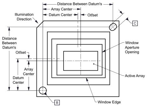
Figure 6. Active Array Location
