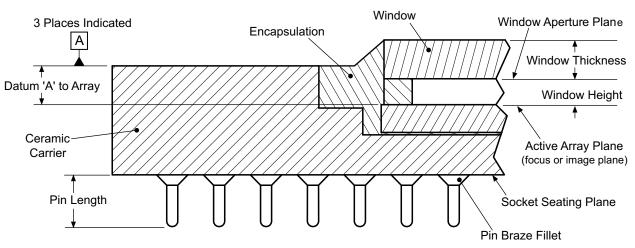
Figure 4. Series-600 DMD Cross Section View
