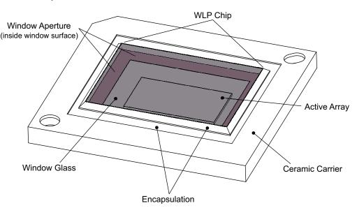
Figure 1. Series-600 DMD Features – Window Side
