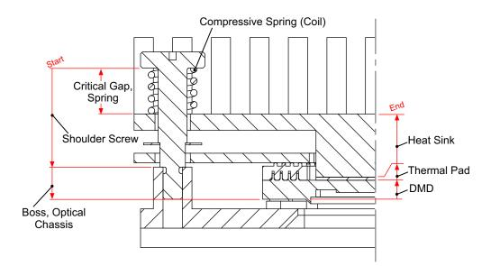
Figure 18. Heat Sink Mounting Tolerance Analysis Schematic Diagram
