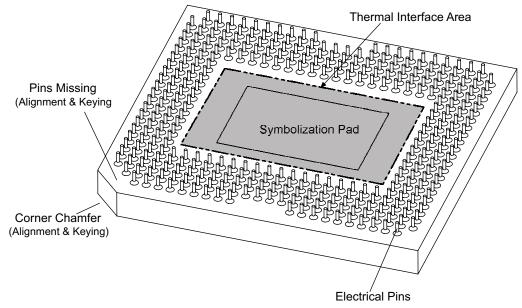
Figure 2. Series-600 DMD Features - Pin Side
