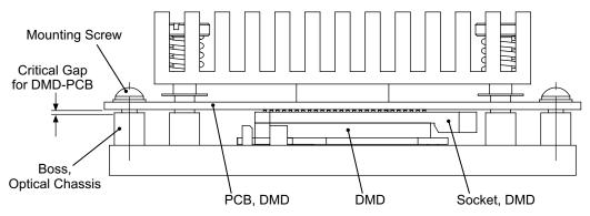
Figure 15. DMD-PCB Mounting Gap - Indirect Control of Load on DMD
