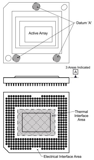
Figure 10. DMD Mechanical Loads
