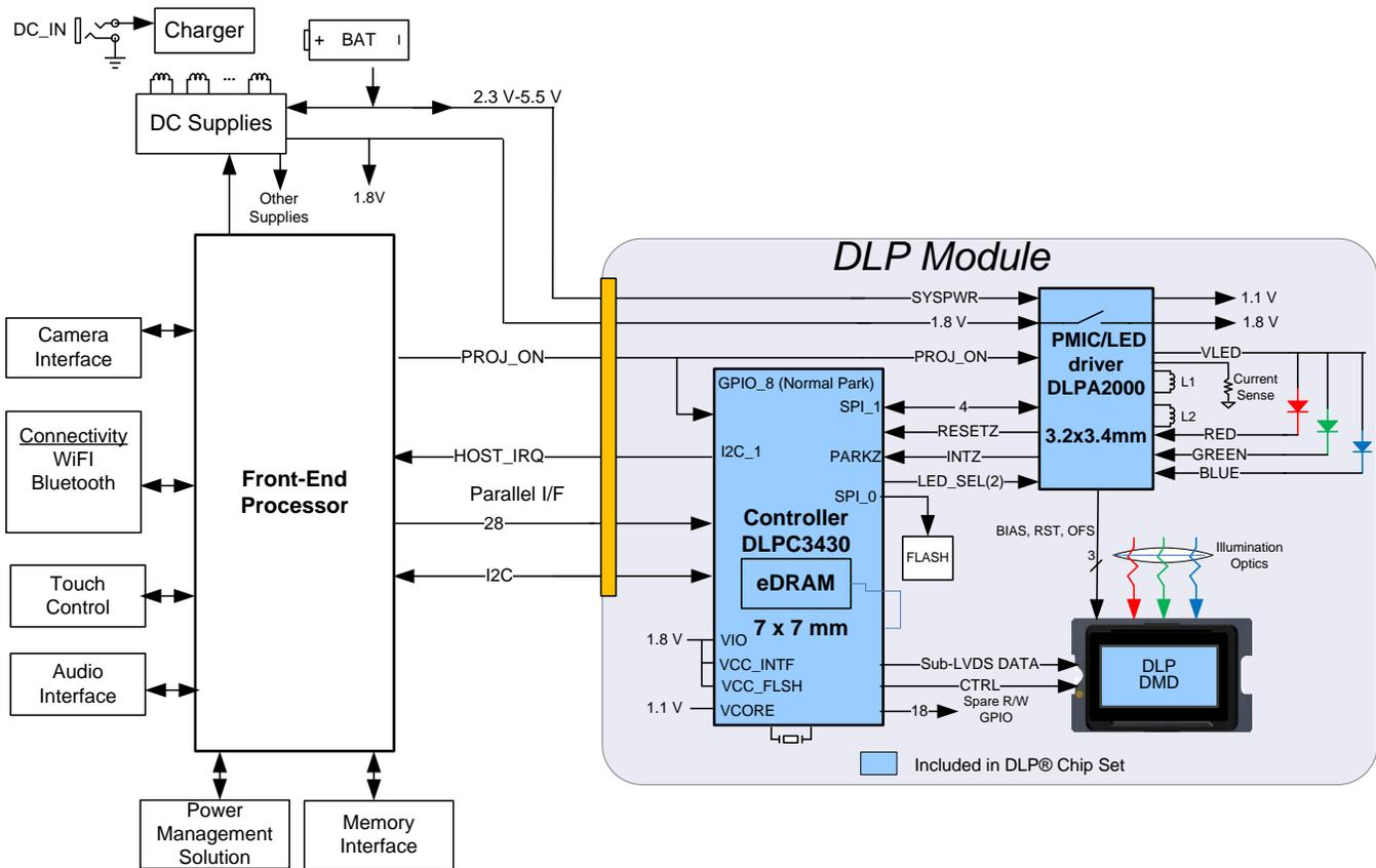
Figure 4-2. Example System Block Diagram
