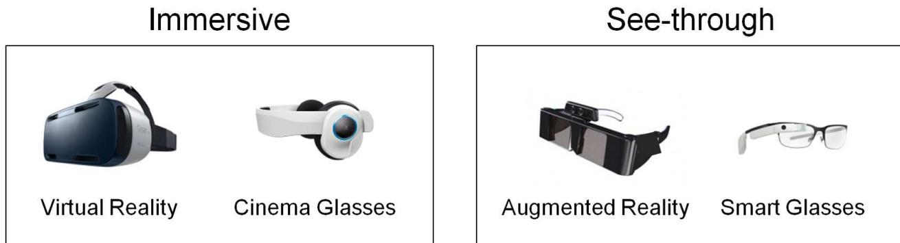
**Figure 2-2. Two General Types of Near Eye Displays**
