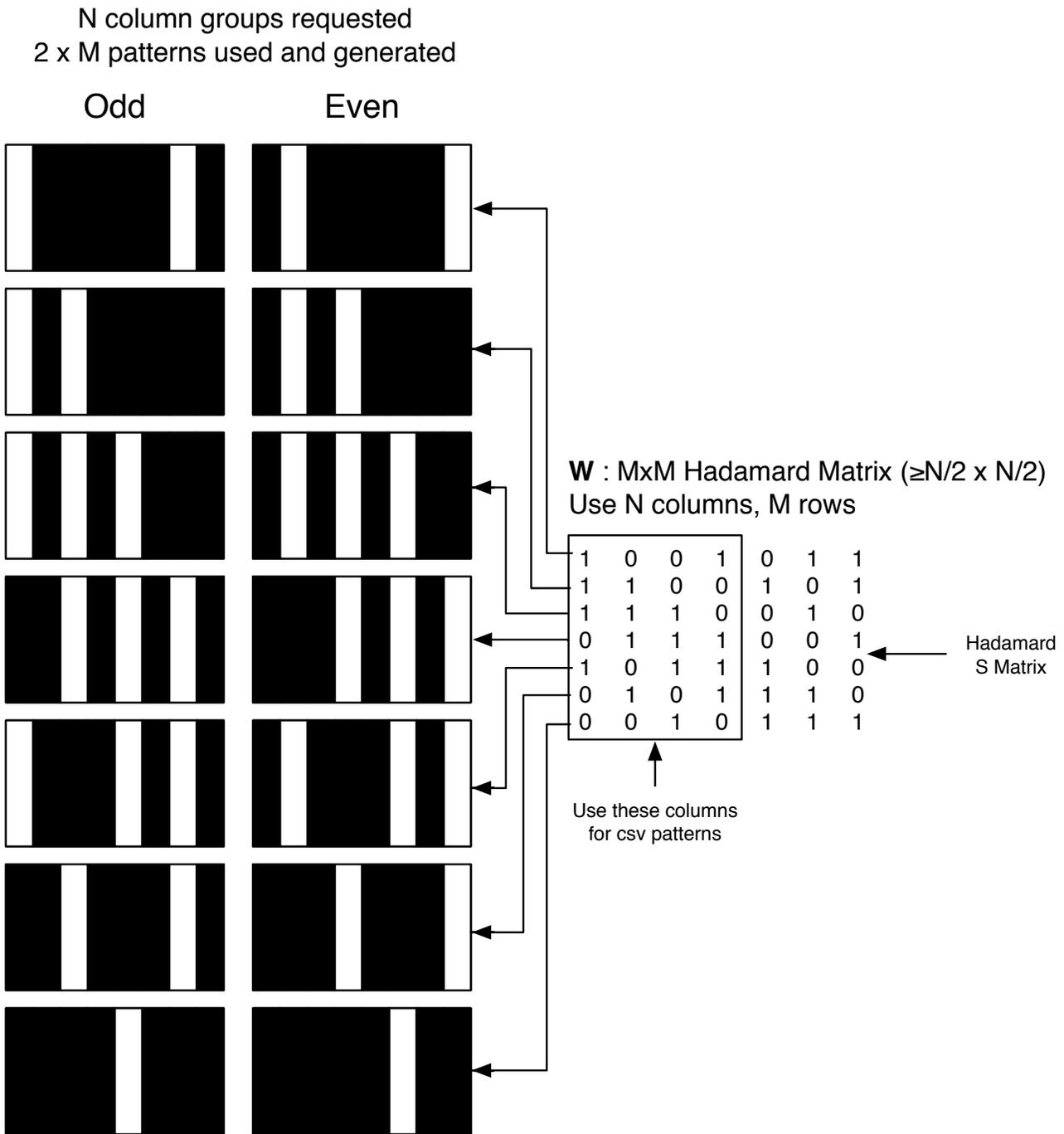
Figure 12. Split Hadamard Scan to Mitigate Diffraction Errors
