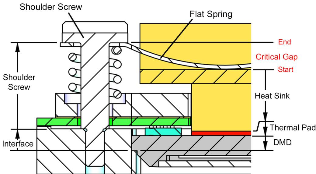
**Figure 20. Flat Spring Gap Tolerance-Analysis Schematic (Shim)**
