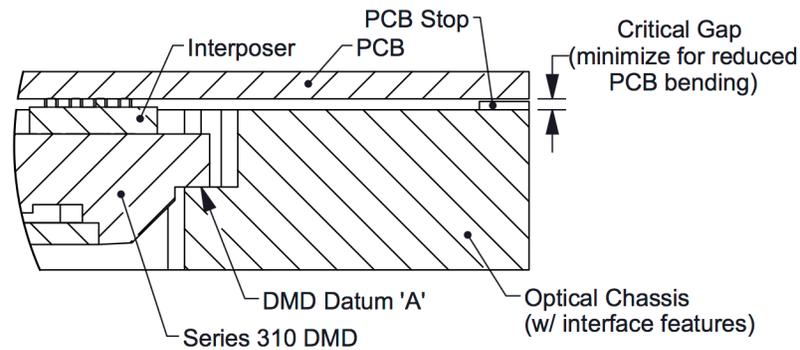
**Figure 12. Mounting Clearance**
