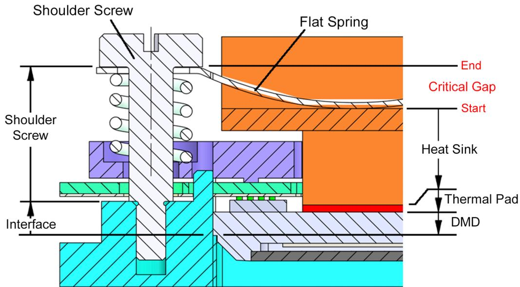
**Figure 25. Flat Spring Gap Tolerance-Analysis Schematic (Clip)**
