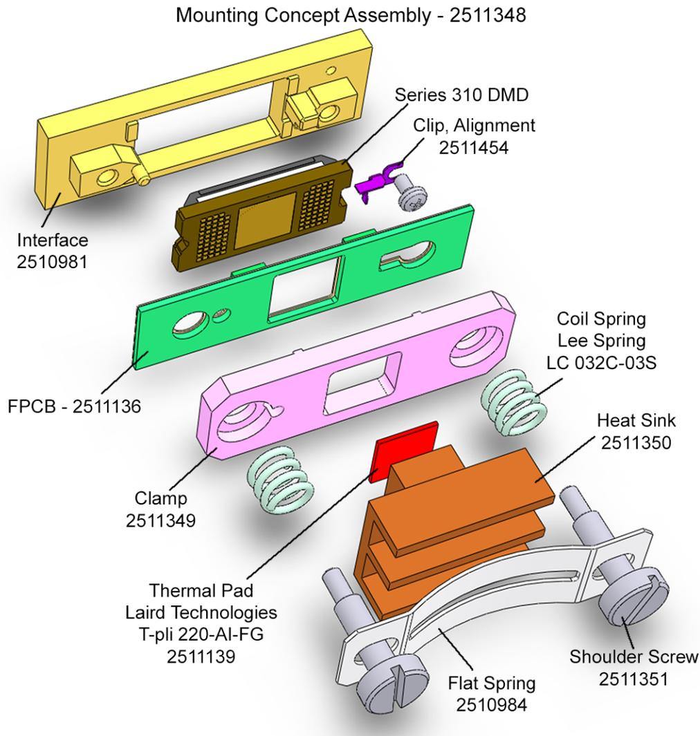
**Figure 23. Clip Alignment Mounting Concept**
