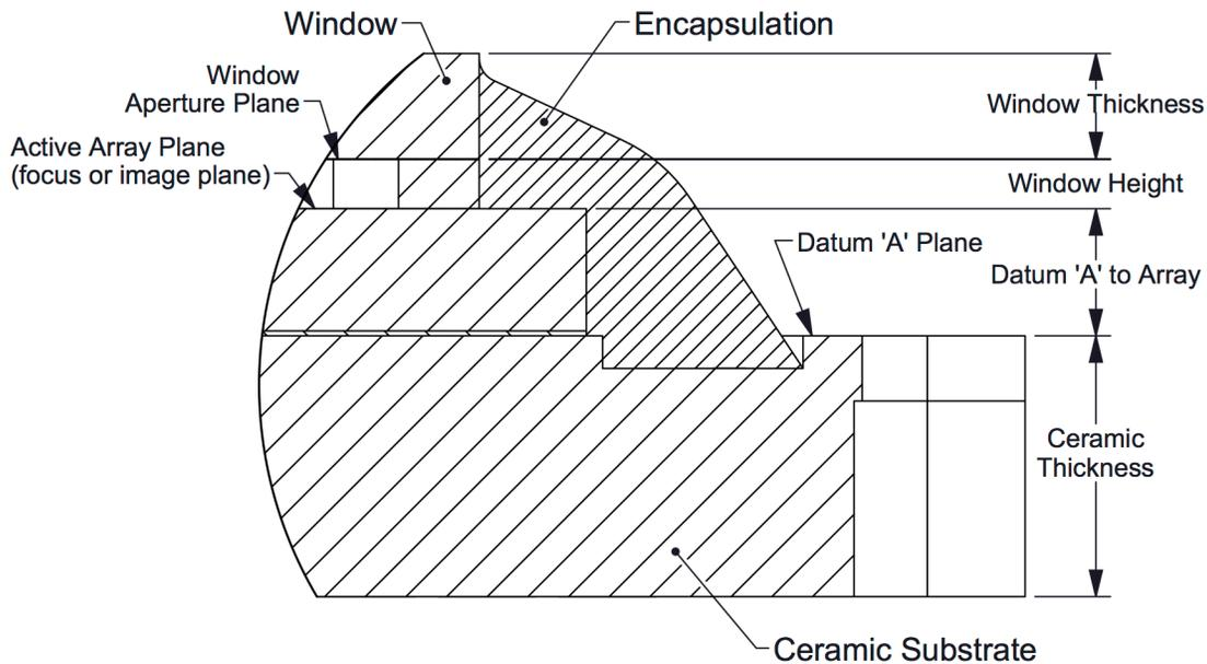
**Figure 4. DMD Cross-Section View Features**
