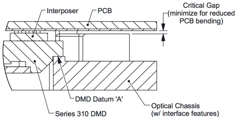
**Figure 13. Mounting Clearance**
