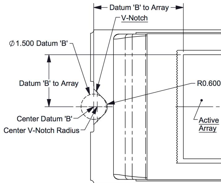
Figure 7. Active Array Location and V-Notch Detail
