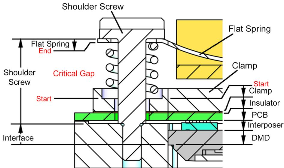
Figure 21. Coil Spring Gap Tolerance-Analysis Schematic (Shim)
