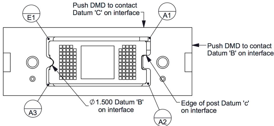
**Figure 14. Mounting Datum 'B' and 'C' Contact**
