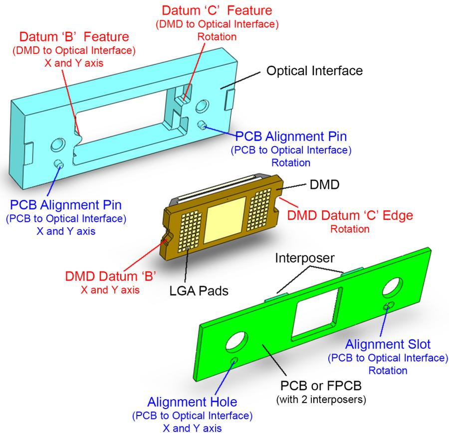
**Figure 15. Electrical Alignment**
