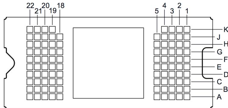
**Figure 9. Pin Numbering Scheme**
