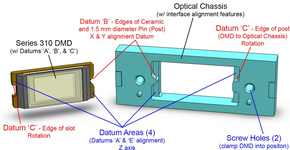
**Figure 11. Optical Interface (Alignment) Features**
