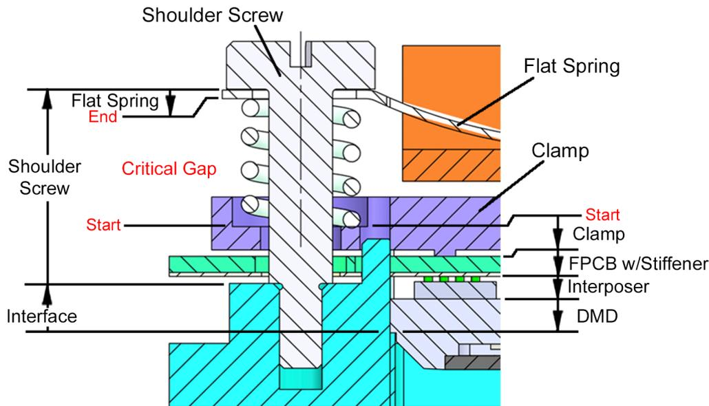
**Figure 26. Coil Spring Gap Tolerance-Analysis Schematic (Clip)**
