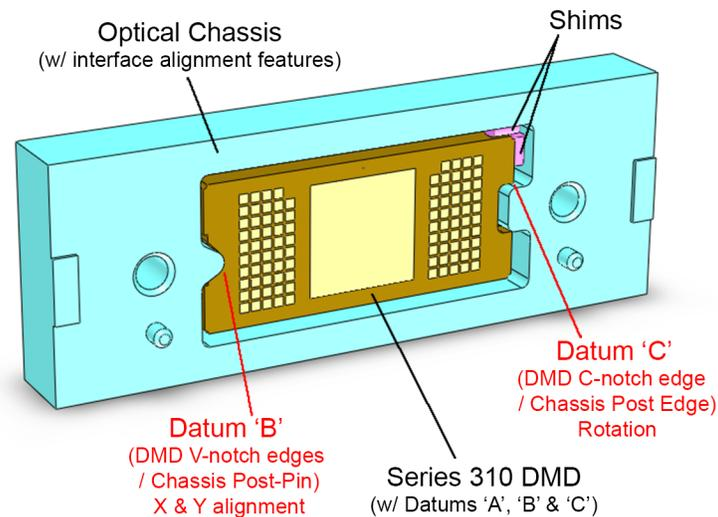
**Figure 18. Alignment Shims**
