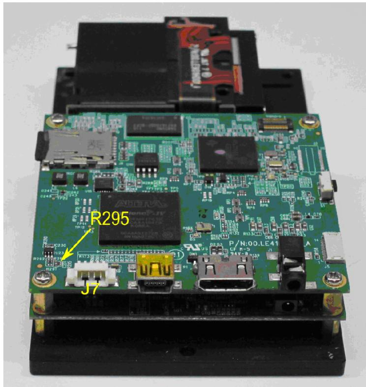
Figure 1. LightCrafter system board, showing location of R295 and J7
