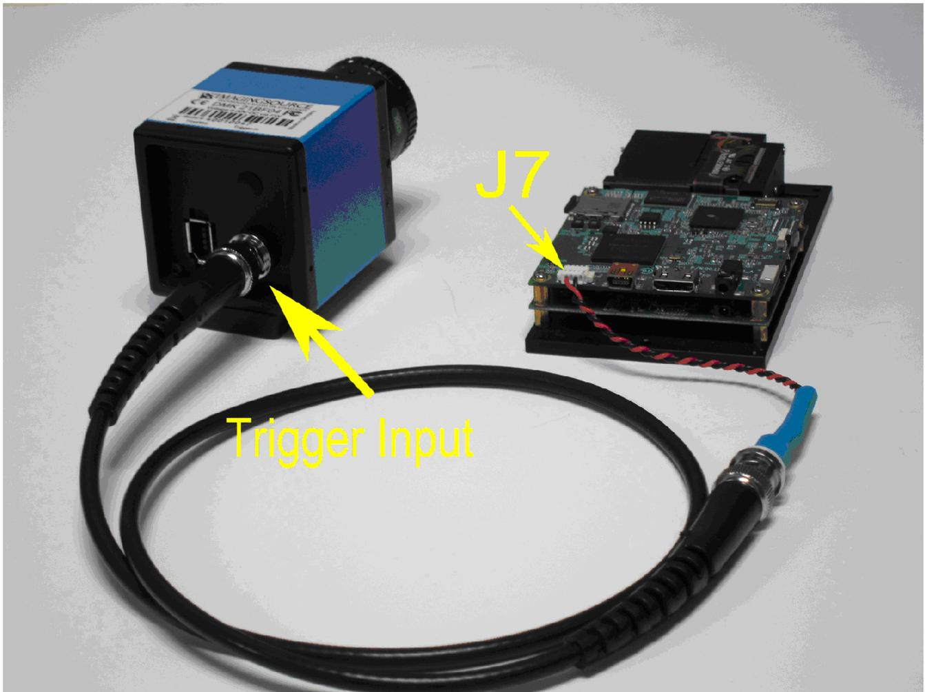
Figure 4. LightCrafter and The Imaging Source camera with trigger cable connected
