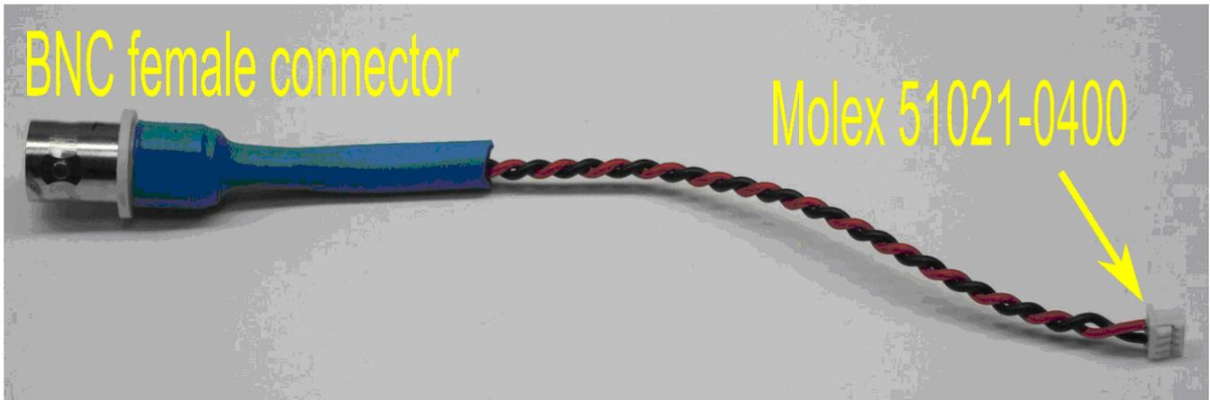
Figure 3. Adapter cable, from LightCrafter J7 to female BNC connector
