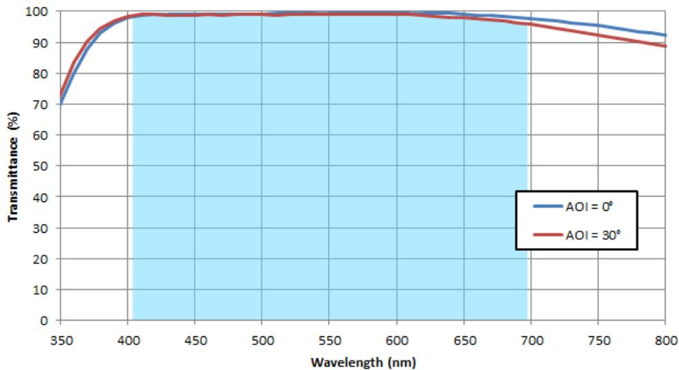
Figure 5. Corning Eagle XG Visible Window Transmittance
