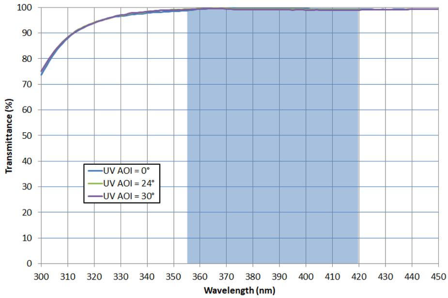
**Figure 3. Corning 7056 UV Window Transmittance (UV Region)**
