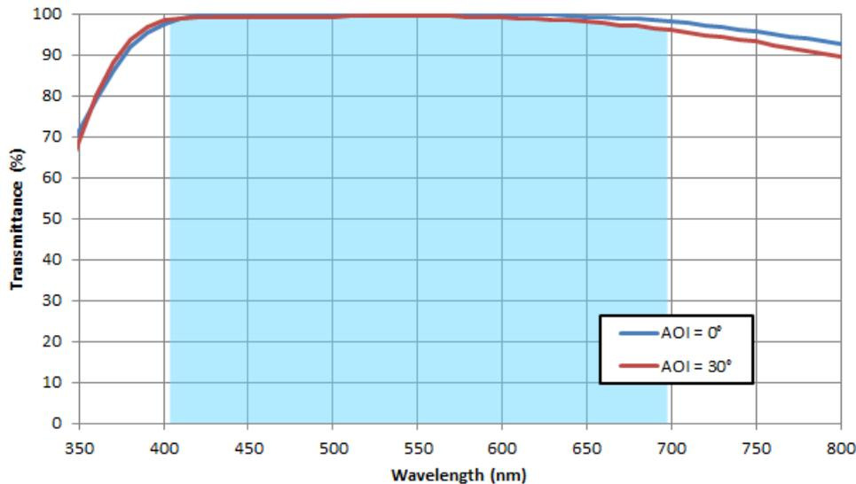
Figure 2. Corning 7056 Visible Window Transmittance (Visible Region)
