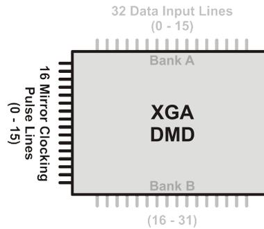
**Figure 4-2. DMD Mirror Clocking Pulse Lines**
