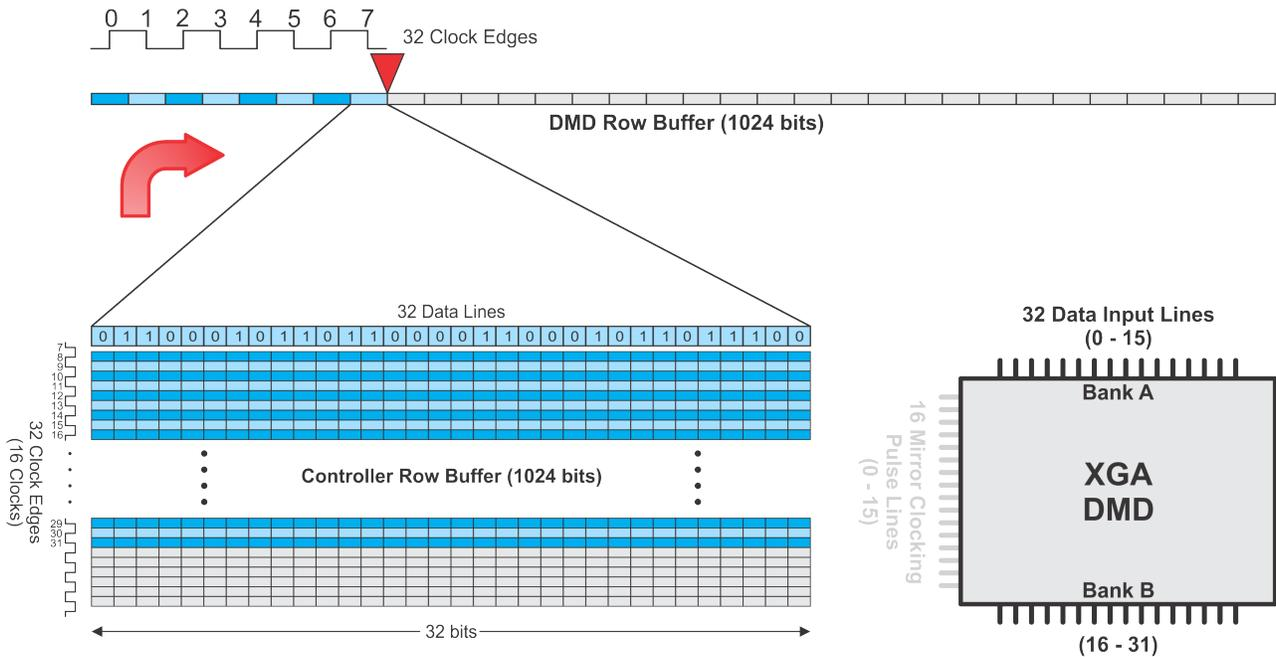
Row data is loaded 32 bits per clock over 32 edges (1024 bits per row) for the 2xLVDS XGA Type A DMD.
