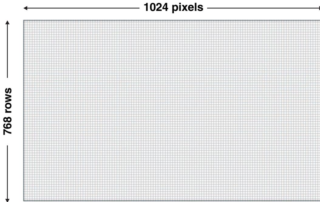
The CMOS memory array consists of 768 rows of 1024 pixels long. 1 = on, 0 = off
