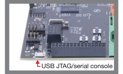
**3** Connect the supplied USB Micro-B to Type-A cable to the microUSB JTAG port J19 and plug the other end into your PC/laptop USB port. Then open a serial console on your PC/laptop such as Teraterm. This cable can also be used for Code Composer Studio (CCS) IDE control of the IDK. Please see [http://processors.wiki.ti.com/index.php/Processor\\_SDK\\_RTOS\\_Setup\\_CCS](http://processors.wiki.ti.com/index.php/Processor_SDK_RTOS_Setup_CCS) for details on CCS set up.
