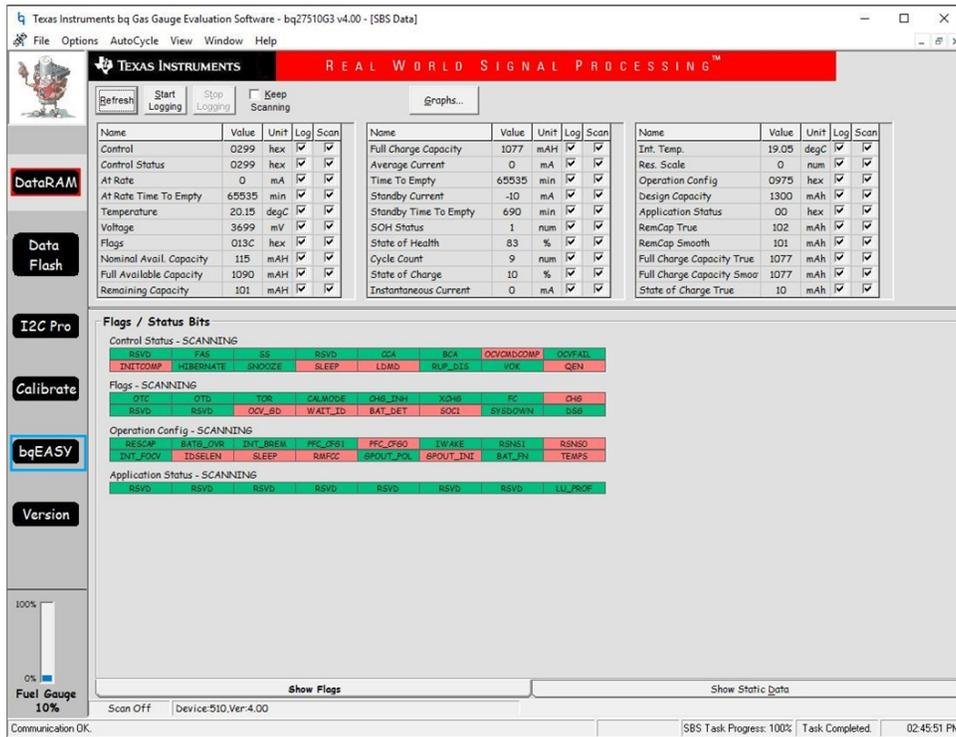
Figure 1-10. bqEVSW Gas Gauge Eval SW DataRam
