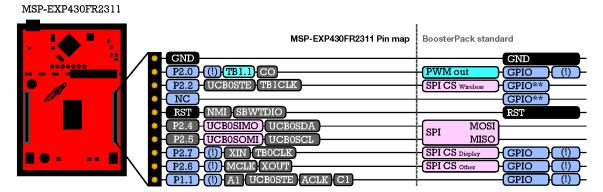
Figure 9. LaunchPad Development Kit To Boosterpack Plug-in Module Connector Pinout
