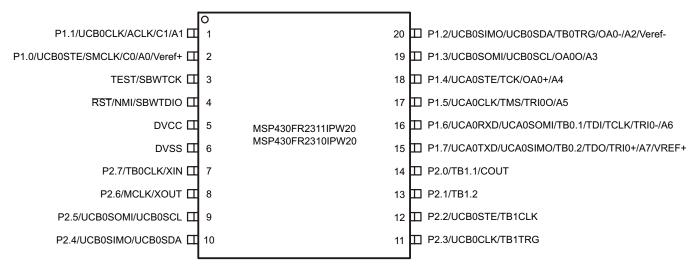
Figure 4. MSP430FR2311 MCU PW20 Pinout
