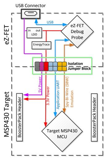
Figure 6. eZ-FET Isolation Jumper Block Diagram
