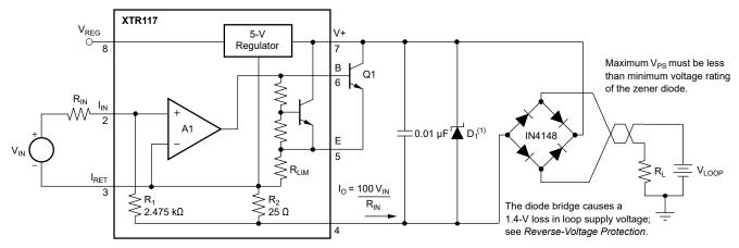
(1) 36-V Zener diode, such as 1N4753A or P6KE39A. Use lower-voltage Zener diodes with loop power-supply voltages < 30 V for increased protection; see Section 6.3.2.
