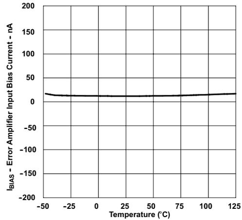
**Figure 7-8. Error Amplifier Input Bias Current vs Temperature**
