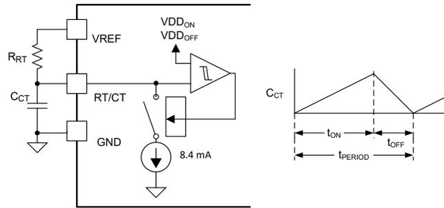
Figure 8-4. Oscillator Circuit
