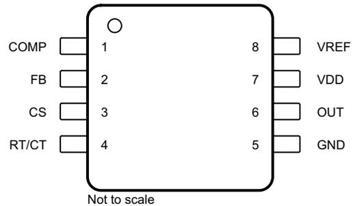
Figure 6-2. DGK Package, 8-Pin VSSOP (Top View)
