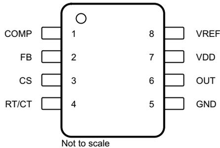
Figure 6-1. D Package 8-Pin SOIC (Top View)
