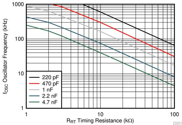
**Figure 7-1. Oscillator Frequency vs Timing Resistance and Capacitance**
