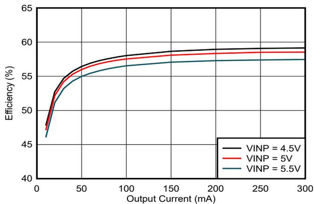
Figure 6-7. Efficiency vs Load Current (I<sub>VCC</sub>): VCC = 5.0V, T<sub>A</sub> = 25°C, C<sub>OUT2</sub> = 22µF
