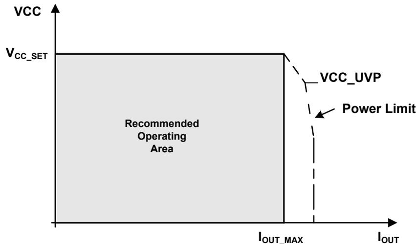
Figure 7-8. VCC Load Recommended Operating Area Description
