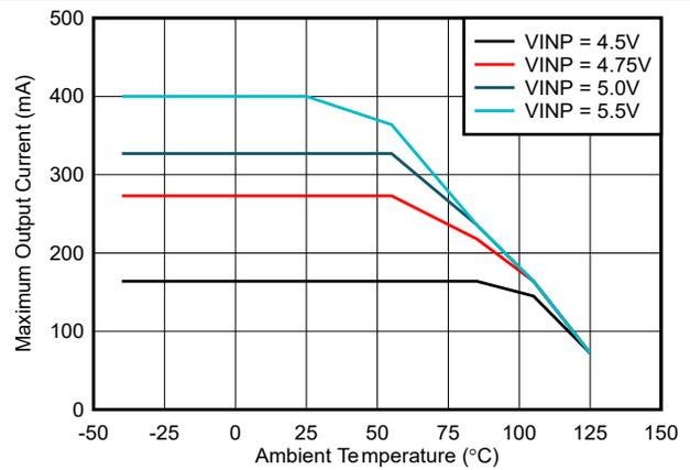
Figure 6-6. Maximum Output Current vs Ambient Temperature :
