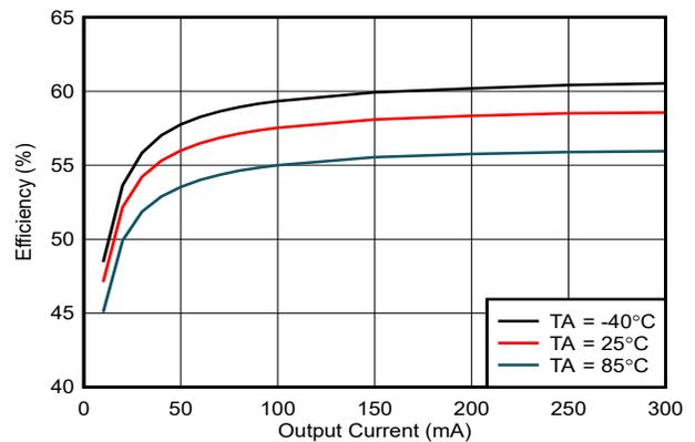
Figure 6-8. Efficiency vs Load Current (I<sub>VCC</sub>): VCC = 5.0V, VINP = 5.0V, C<sub>OUT2</sub> = 22µF
