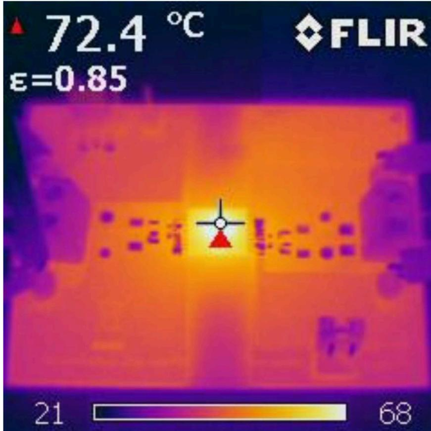
Figure 8-8. UCC33421-Q1 Thermal Image: VINP = 5.0V, VCC = 5.0V, P<sub>Out</sub>=1.5W
