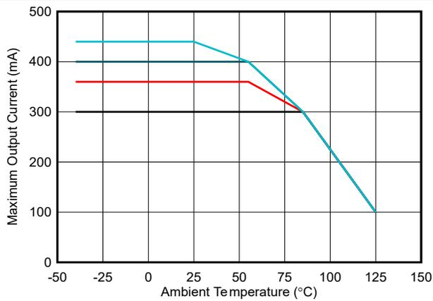
Figure 6-5. Maximum Output Current vs Ambient Temperature :
