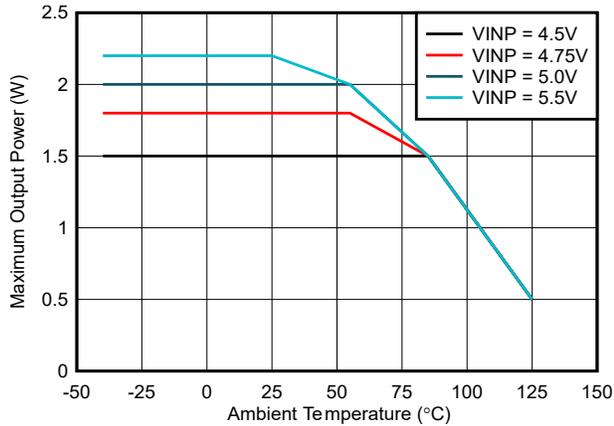
Figure 6-3. Maximum Output Power vs Ambient Temperature :
