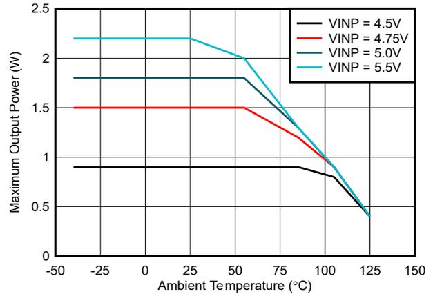
Figure 6-4. Maximum Output Power vs Ambient Temperature :
