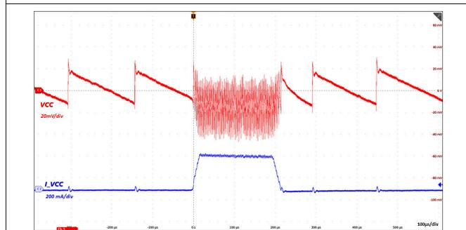
**Figure 8-4. Load Transient: VINP = 5.0V, VCC = 5.0V, C<sub>OUT2</sub> = 22µF, I<sub>VCC</sub> = 0mA - 300mA - 0mA**
