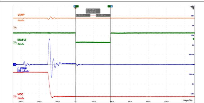
**Figure 8-5. Output Short Circuit Operation: VINP = 5.0V**
