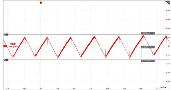
Figure 6-14. Steady State Output Voltage Ripple: VINP = 5.0V, VCC = 5.0V, 300mA Load
