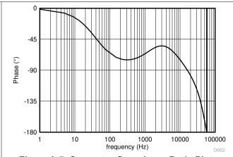
Figure 9-5. Converter Open-Loop Bode Plot -Phase
