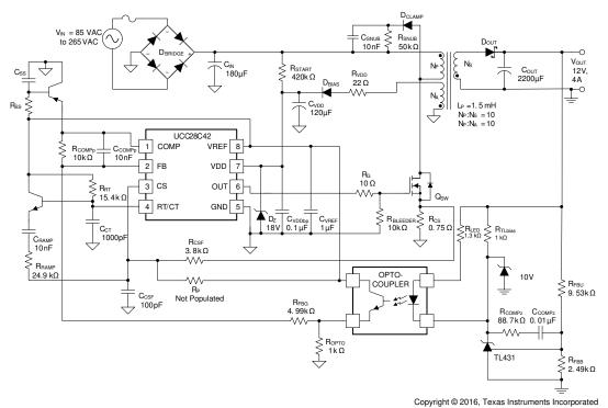
Figure 9-3. Typical Application Design Schematic
