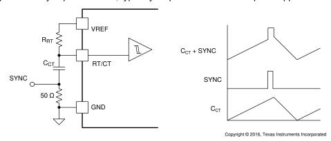
Figure 8-5. Oscillator Synchronization Circuit
