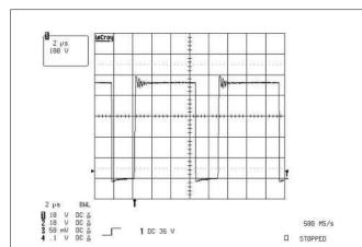
Figure 9-8. Primary Side MOSFET Drain to Source Voltage at 240-V AC Input (100 V/div)
