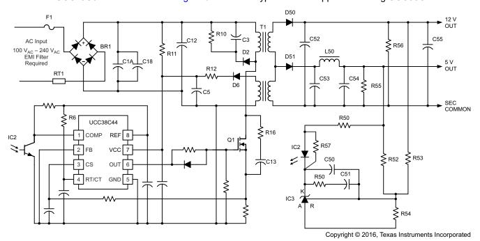
Figure 9-1. Typical Off-Line Application
