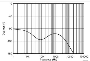
Figure 9-7. Converter Closed-Loop Bode Plot – Phase
