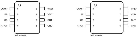
Figure 6-1. D Package 8-Pin SOIC (Top View)
