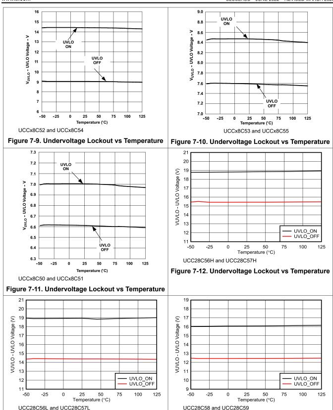
Figure 7-13. Undervoltage Lockout vs Temperature | Figure 7-14. Undervoltage Lockout vs Temperature
