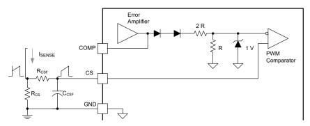
Figure 8-3. Current-Sense Circuit Schematic
