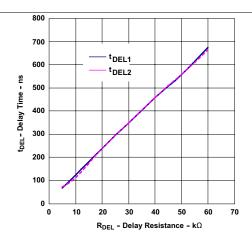
Figure 15. Delay Time vs. Delay Resistance
