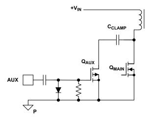
Figure 24. Low-Side P-Channel
