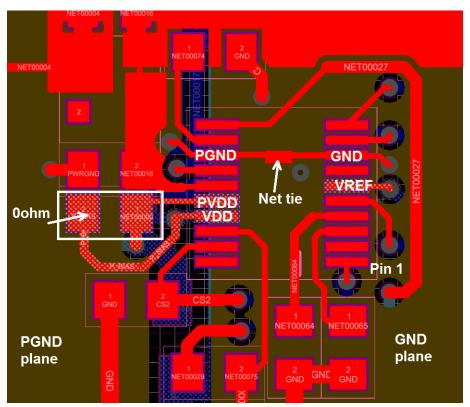
Figure 33. Layout Example Top Layer
