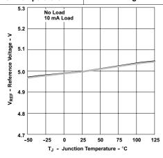
Figure 18. Reference Voltage vs. Temperature
