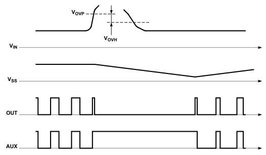
Figure 21. Line Overvoltage Sequence, P-Channel
