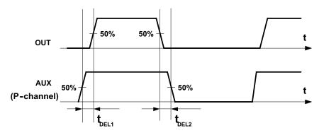
Figure 1. Output Timing Diagram
