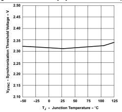
Figure 13. Synchronization Threshold Voltage vs. Junction Temperature
