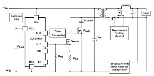
Figure 29. Active Clamp Forward Converter
