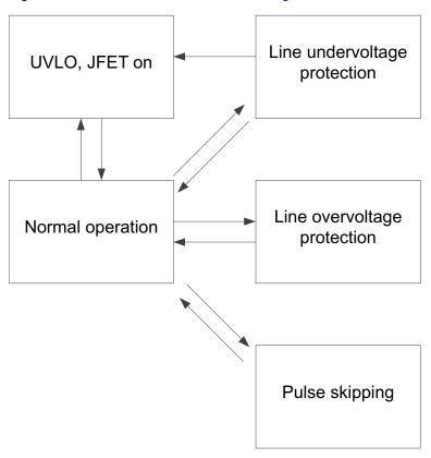
Figure 27. Mode Transition Diagram
