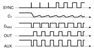
Figure 23. A Synchronization Waveform for SYNC Input, P-Channel
