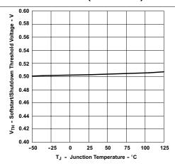
Figure 8. Soft Start/Shutdown Threshold Voltage vs. Junction Temperature
