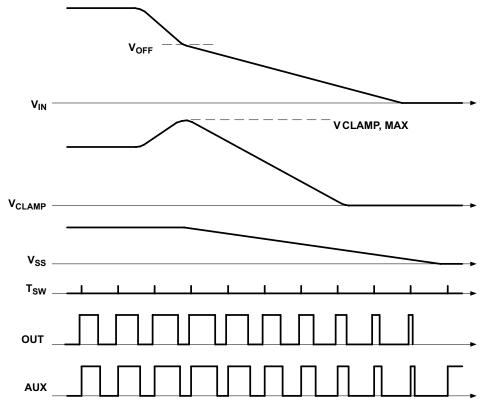
Figure 20. Line Undervoltage Shutdown Waveforms, P-Channel
