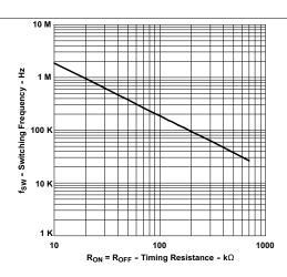
Figure 9. Switching Frequency vs. Programming Resistance
