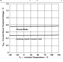
Figure 12. Current Sense Threshold Voltage vs. Junction Temperature
