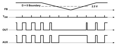
Figure 22. Pulse Skipping Operation, P-Channel
