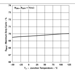
Figure 11. Maximum Duty Cycle vs. Junction Temperature
