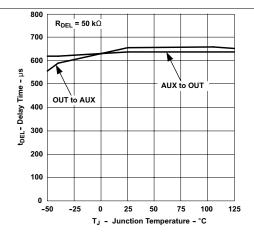
Figure 17. Delay Time vs. Junction Temperature
