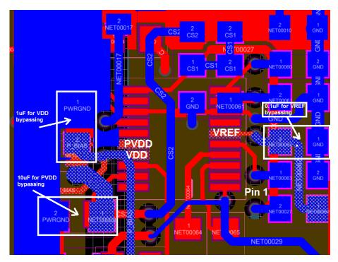
Figure 34. Layout Example Bottom Layer
