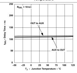
Figure 16. Delay Time vs. Junction Temperature
