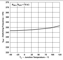
Figure 10. Oscillator Frequency vs. Junction Temperature
