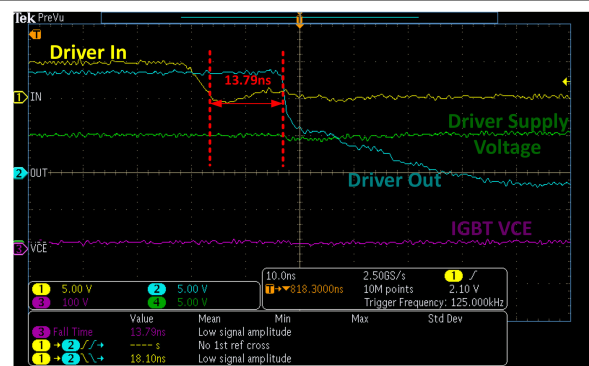
Figure 7-3. UCC27624-Q1 Used to Drive IGBT in the Boost Converter
