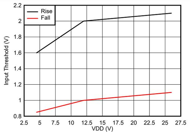
Figure 5-8. Input Thresholds
