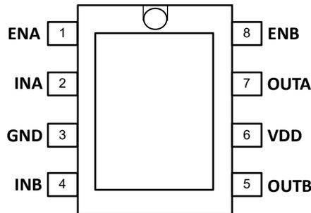
Figure 4-5. DDA Package 8-Pin SOIC Top View
