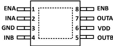
Figure 4-2. DGN Package 8-Pin VSSOP Top View
