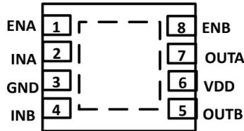
Figure 4-3. DSD Package 8-Pin WSON Top View
