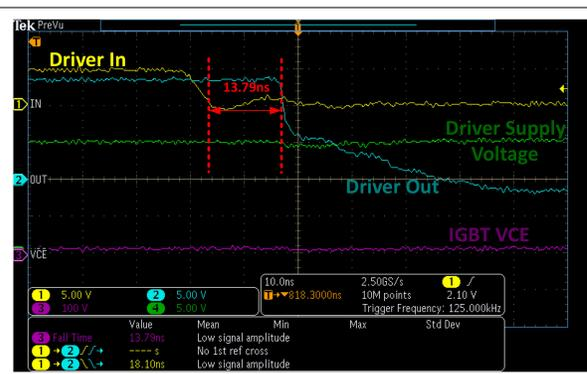
Vin = 210 V, Vout = 235 V, Iout = 1.14 A, Fsw = 100 kHz,
