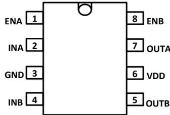
Figure 4-1. D Package 8-Pin SOIC Top View
