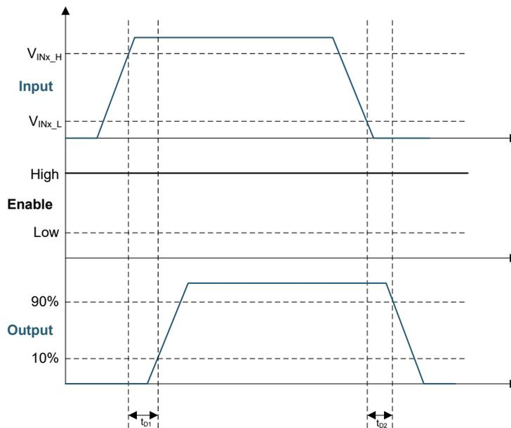
Figure 5-2. Input-Output Operation
