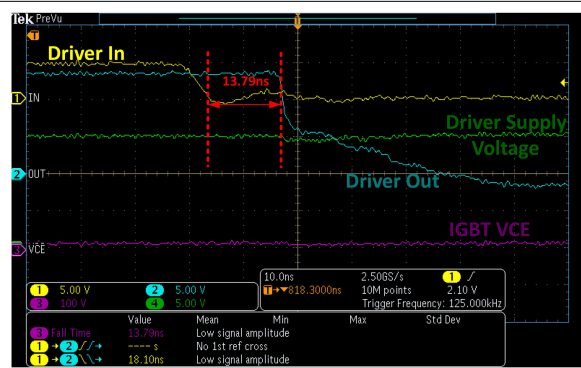
Figure 8-3. UCC27524A1-Q1 Used to Drive IGBT in the Boost Converter
