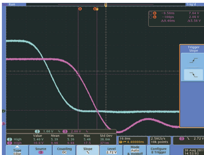
Figure 25. Typical Turn-On Waveform (VDD = 10 V, CL = 1 nF)
