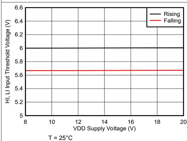
Figure 5-6. UCC27200A Input Threshold vs Supply Voltage
