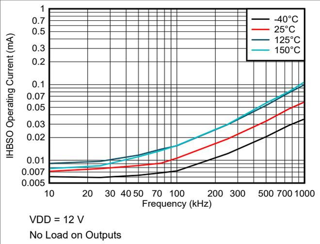
Figure 5-5. HB to VSS Operating Current vs Frequency
