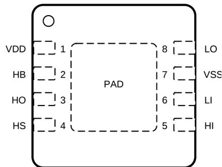
Figure 4-3. DRM Package 8-Pin VSON Top View
