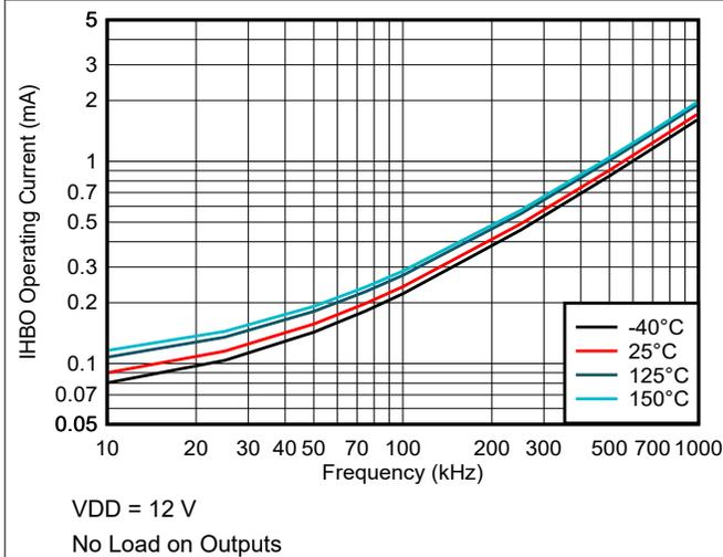
Figure 5-4. Boot Voltage Operating Current vs Frequency
