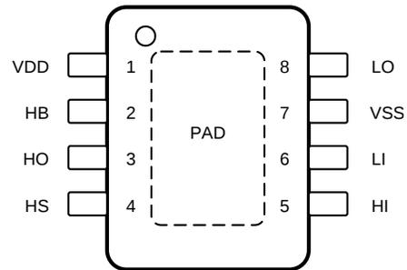
Figure 4-2. DDA Package 8-Pin SO PowerPAD Top View
