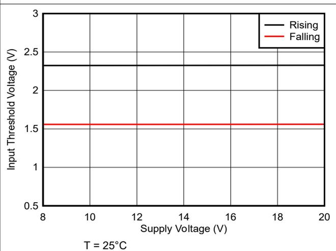
Figure 5-7. UCC27201A Input Threshold vs Supply Voltage
