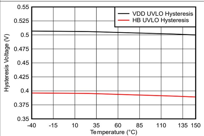
Figure 5-13. Undervoltage Lockout Threshold Hysteresis vs Temperature
