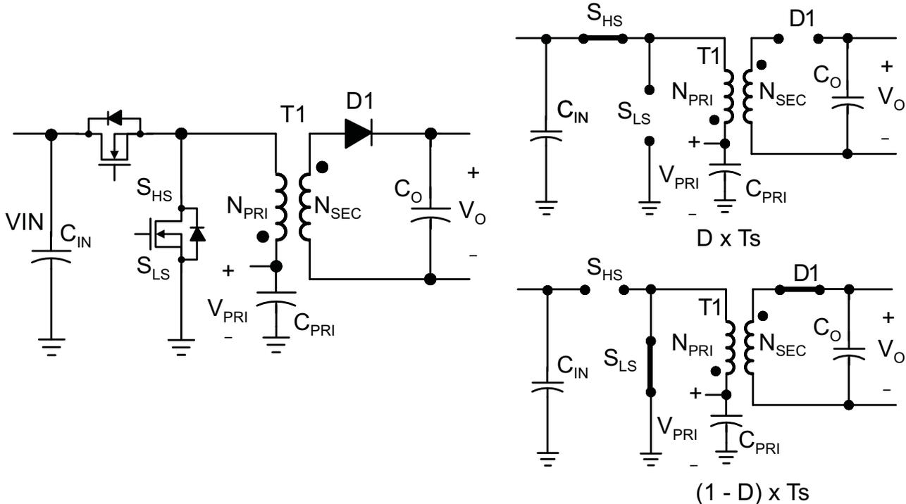
Figure 7. Simplified Schematic with Two Primary Operational States
