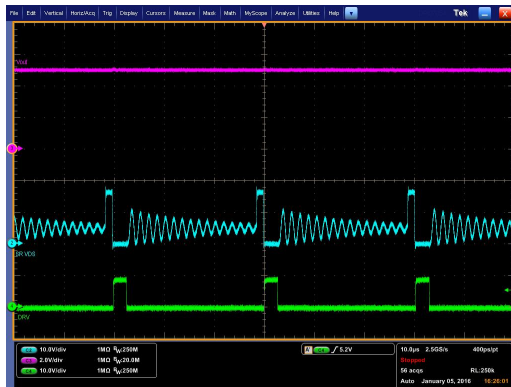
CH2 (Blue): Drain of synchronous rectifier Q1, 10V/Div CH3 (Magenta): V_{OUT} , 2V/Div CH4 (Green): DRV signal to Q1, 10V/Div
