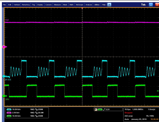
CH2 (Blue): Drain of synchronous rectifier Q1, 10V/Div CH3 (Magenta): V_{OUT} , 2V/Div CH4 (Green): DRV signal to Q1, 10V/Div
