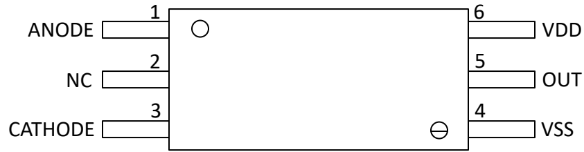
Figure 4-1. UCC23525 DWY Package SO-6 Top View
