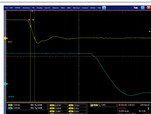
Figure 9-13. PWM Input (yellow) and Driver Output (blue) Falling Edge
