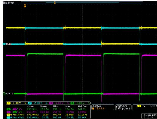
Figure 8-5. Bench Test Waveform for INA/B and OUTA/B
