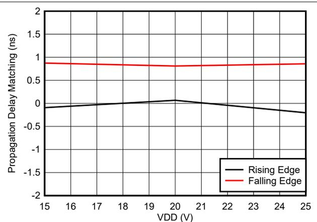
Figure 5-19. Propagation Delay Matching (t<sub>DM</sub>) vs VDD
