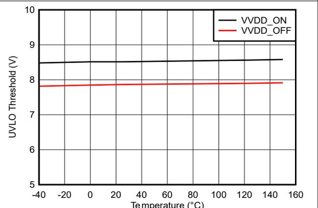
**Figure 5-23. VDD 8-V UVLO Threshold vs Temperature**
