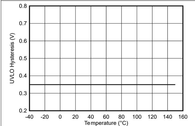
**Figure 5-22. VDD 5-V UVLO Hysteresis vs Temperature**
