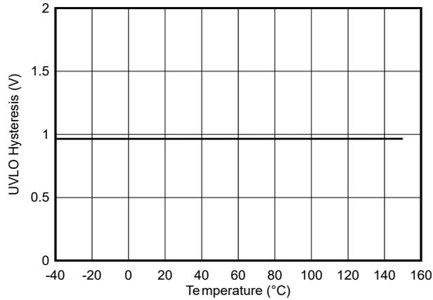
Figure 5-26. VDD 12-V UVLO Hysteresis vs Temperature
