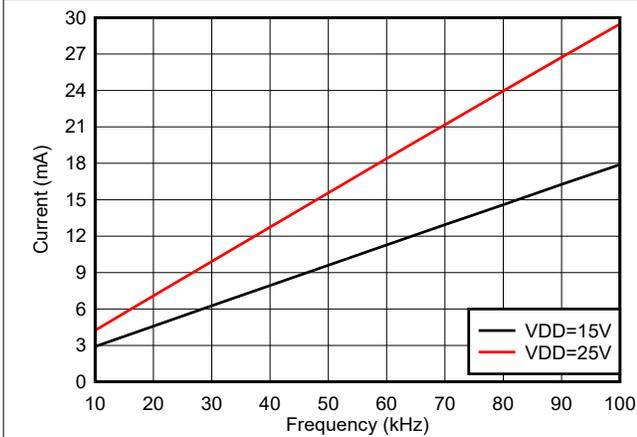
Figure 5-10. Per Channel Current Consumption ( $I_{VDDA/B}$ ) vs Frequency (10-nF Load, VDD = 15 V or 25 V)
