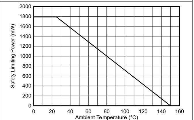
**Figure 5-4. Thermal Derating Curve for Safety-Related Limiting Power per VDE for DW Package**
