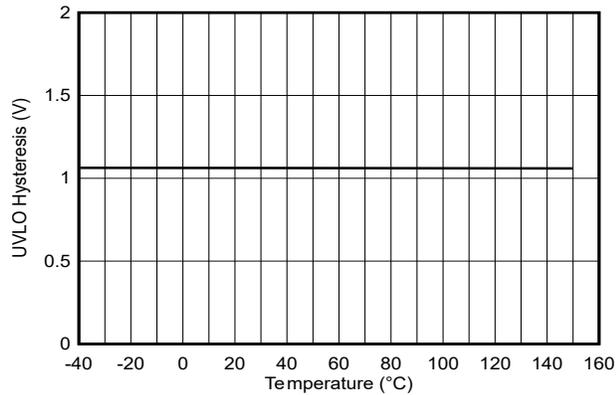
Figure 5-28. VDD 17-V UVLO Hysteresis vs Temperature
