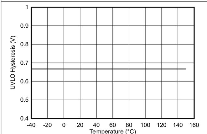
**Figure 5-24. VDD 8-V UVLO Hysteresis vs Temperature**
