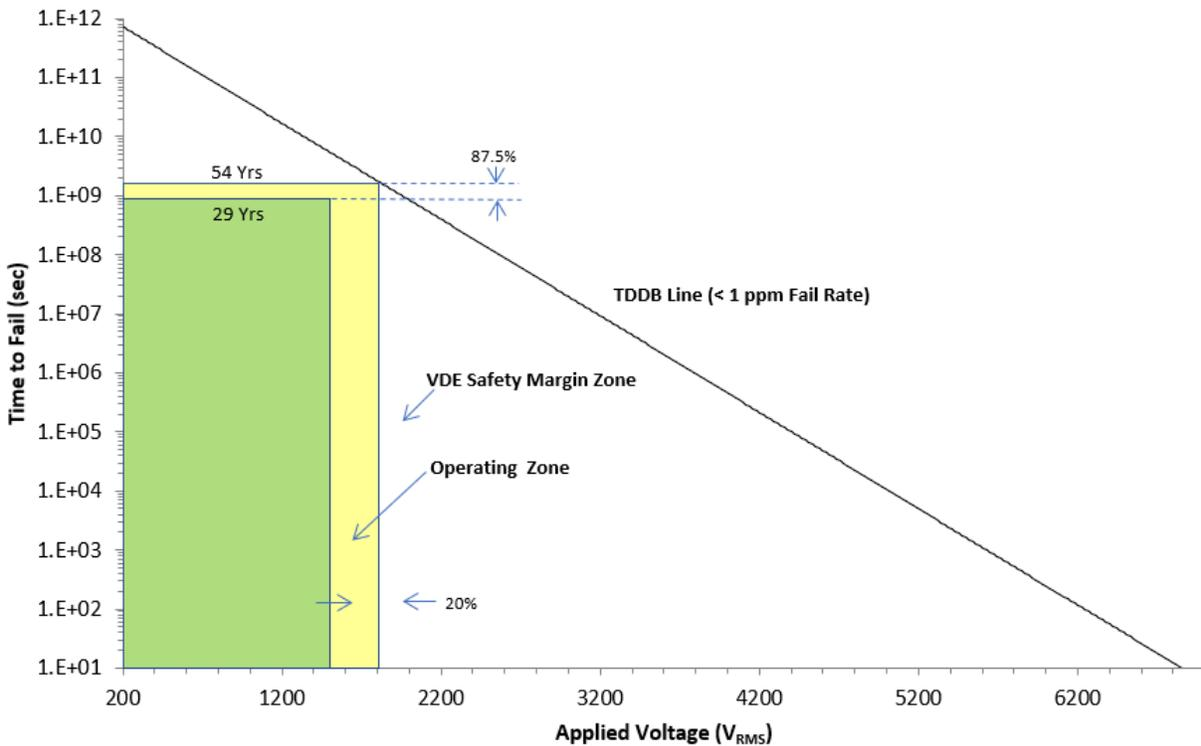
Working Isolation Voltage = 1500 V<sub>RMS</sub>
