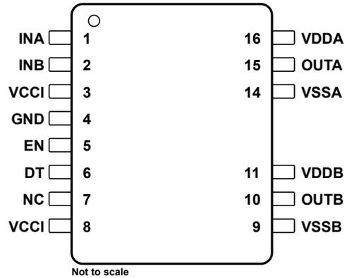
Figure 4-2. DWK Package 14-Pin SOIC Top View
