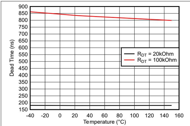
Figure 5-32. Dead Time vs Temperature (with R<sub>DT</sub> = 20 kΩ and 100 kΩ)
