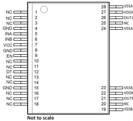
Figure 4-3. DFJ Package 28-Pin SOIC Top View
