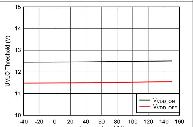
**Figure 5-25. VDD 12-V UVLO Threshold vs Temperature**
