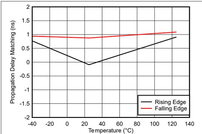
**Figure 5-20. Propagation Delay Matching (t<sub>DM</sub>) vs Temperature**
