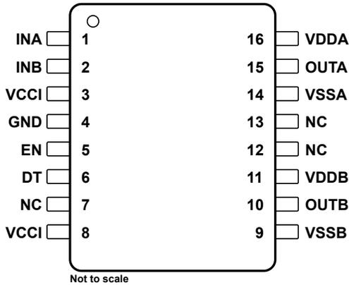
Figure 4-1. DW Package 16-Pin SOIC Top View
