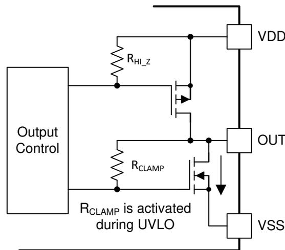
**Figure 7-1. Simplified Representation of Active Pulldown Feature**
