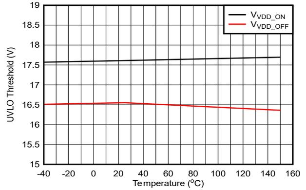
Figure 5-27. VDD 17-V UVLO Threshold vs Temperature
