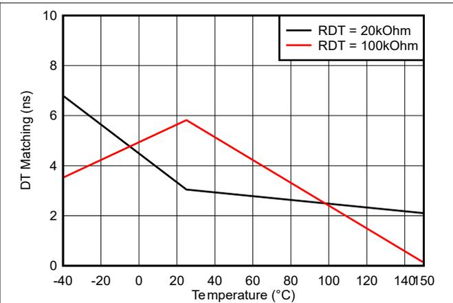
Figure 5-33. Dead Time Matching vs Temperature (with R<sub>DT</sub> = 20 kΩ and 100 kΩ)
