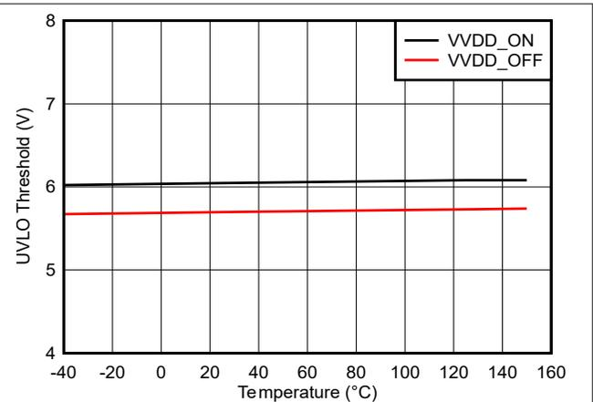
**Figure 5-21. VDD 5-V UVLO Threshold vs Temperature**
