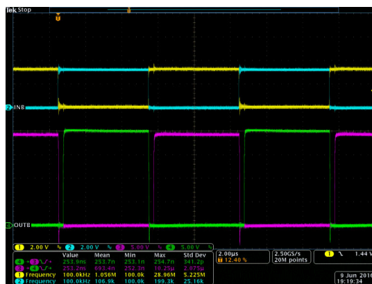
Figure 8-5. Bench Test Waveform for INA/B and OUTA/B
