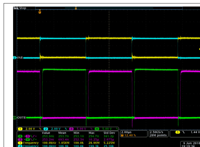
Figure 9-5. Bench Test Waveform for INA/B and OUTA/B
