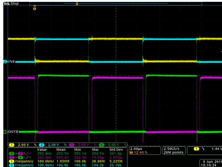
Figure 8-5. Bench Test Waveform for INA/B and OUTA/B
